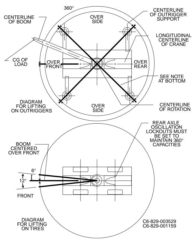
BOLD LINES DETERMINE THE LIMITING POSITION OF ANY LOAD FOR OPERATION WITHIN WORKING AREAS INDICATED
