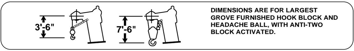
DIMENSIONS ARE FOR LARGEST GROVE FURNISHED HOOK BLOCK AND HEADACHE BALL, WITH ANTI-TWO BLOCK ACTIVATED.
