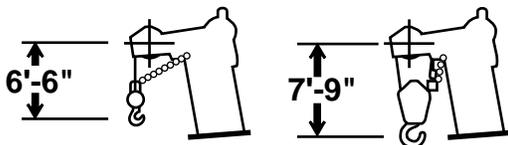
DIMENSIONS ARE FOR LARGEST GROVE FURNISHED HOOK BLOCK AND HEADACHE BALL, WITH ANTI-TWO BLOCK ACTIVATED.
