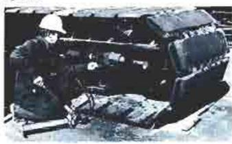
CRAWLER SPROCKET AND TUMBLER: Durable steel casting with flame-hardened teeth and nm. Mounted on stationary shaft supported at both ends by crawler frame for maximum etrength and proper elignment. Sprocket and tumbler revolve on two bronze bushings lubricated by center grease pocket for efficient operation. Self-cleaning tumbler has alternate sides open.
