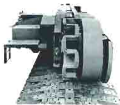
CRAWLER GEAR AND TUMBLER: Transmit drive torque. Cast steel with a large bushing on each end and a grease pocket in center. Mounted on stationary shaft which is supported at both ends in the side frame. Tumbler is of self-cleaning design with alternate sides open.
