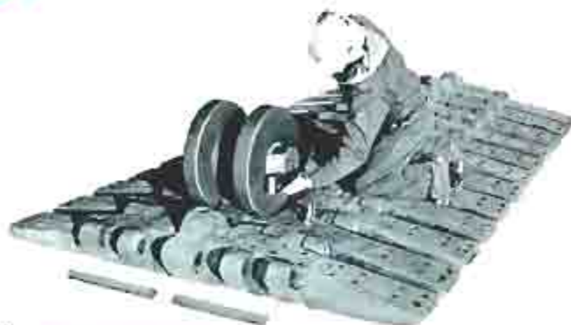
CRAWLER TREADS: 83 inches wide, constructed of cast alloy steel closed box section design with large center driving lug. 77 treads per crawler side frame. Each pad connected by two high carbon steel pins.
