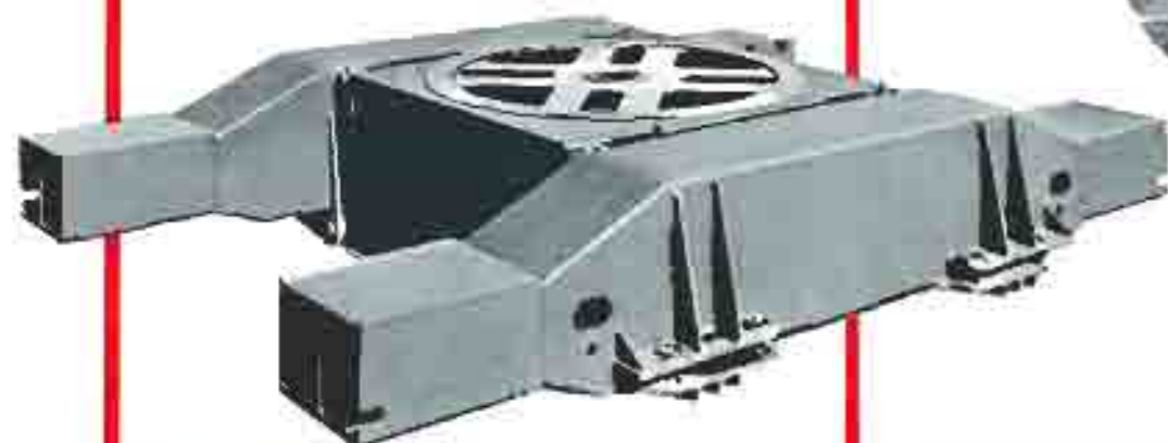
TRANSVERSE BEAMS: Two fabricated beams pin connect to carbody. The beam ends form wings to receive crawler frames on large machined surfaces.
