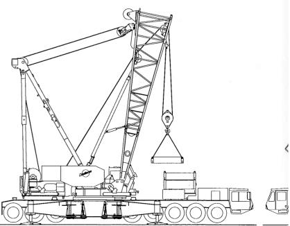
**Step 6:** Counterweight is removed from trailers and assembled atop carrier.
