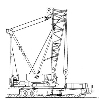
**Step 5:** Gantry is pulled into upright position with boom hoist and secured by power-activated backhitch pins. Outriggers are removed from trailer and attached to carrier using FACT system of pin connections.
