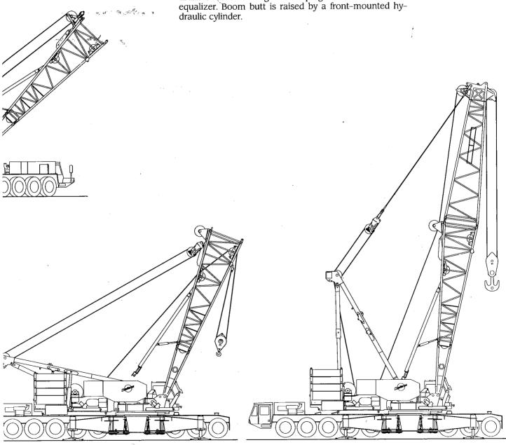
**Step 7:** Gantry is lowered. Counterweight is pendant-connected to gantry; raised into position using counterweight-raising cylinders; and attached to upperworks by power-activated pins.
