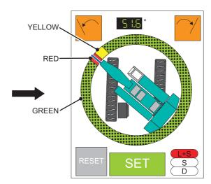
(C) Swing the crane to the place just before the obstacle on the right side and stop and push the icon [RIGHT LIMIT POSITION SET].
