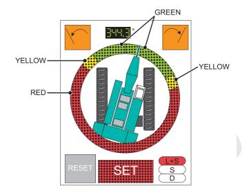
(B) To set again, push [RESET] icon. The screen returns to the one shown right. Set again based on new setting procedure (P.3-54).
