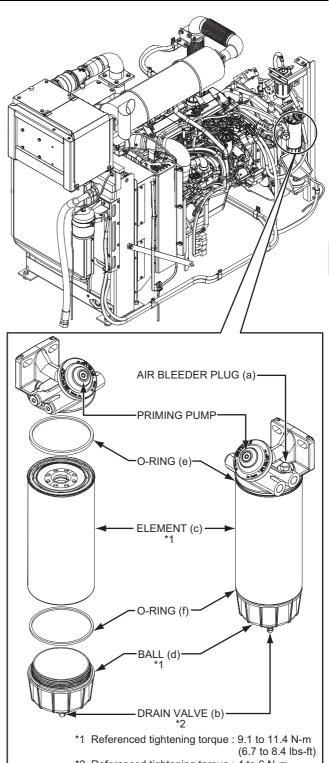
\*2 Referenced tightening torque : 4 to 6 N-m (3 to 4.4 lbs-ft)
