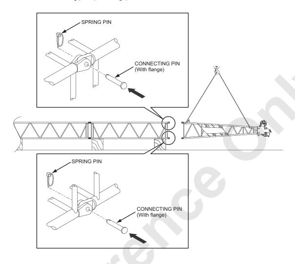
As an alternative way of attachment connection, the boom inserts and boom top are to be connected first and then the boom base and the boom inserts can be connected as last as shown below.
