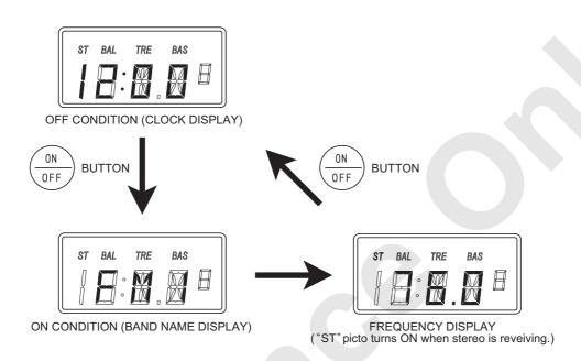
Under this condition, by pressing "Display select" button (frequency/clock), frequency display and clock display alternates.
