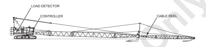
7. Referring to chapter "3. LOAD SAFETY DEVICE", input the crane configuration data in the load safety device.
