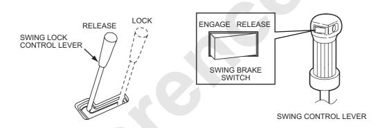
3. Push the swing control lever forward to swing the upper to the left and pull the lever backward to swing the upper to the right.
