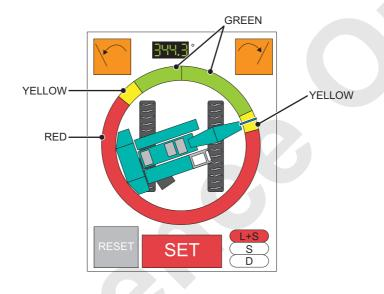
(4) If the crane continues to swing further and the front of the boom enters into red area on circle, continuous warning sound is issued and swing motion stops.
