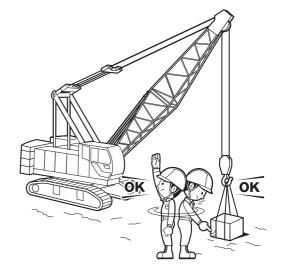
21. If there is not enough wire rope on the drum the rope can snap loose.
