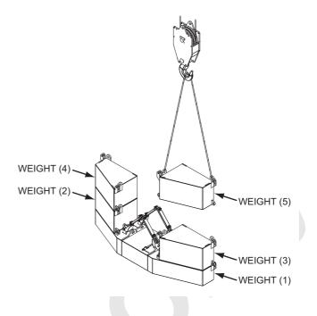
6. Secure right and left counterweights with the connecting pins respectively and retain them with the spring pins. (8 locations)
