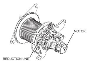
FRONT, REAR DRUM MOTOR AND REDUCTION UNIT
