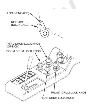
These knobs are to lock the drum to for safety during lowering the lifting load or boom.
