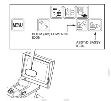
5. By lowering the boom further, the hook overhoist limit switch operates when the weight of the hook overhoist limit switch is placed on the ground, and the boom lowering is automatically stopped again. Press and hold the "Assy/disassy" icon one time for approx. 1 second and it becomes the Assy/disassy mode, and the boom can be lowered. Be careful because the hook overhoist automatic stop does not function in the Assy/disassy mode.
