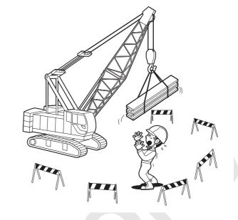
10. Rapid swings or sudden starts and stops can cause the hook and attached load to swing out of control. Always start and stop movements smoothly and swing at speeds that will keep the load under control.
