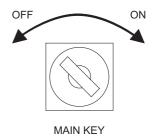
LOAD SAFETY DEVICE BYPASS CONFIGURA-TION SELECT SWITCH
