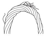
Bend rope sharply to expose breakage.
