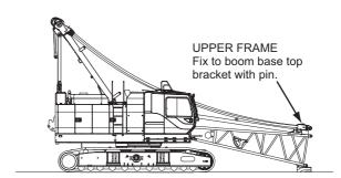
Turn the boom drum control lever to lowering side and pay out the boom hoist wire rope slowly until the ropes are placed on the boom base and the gantry.
