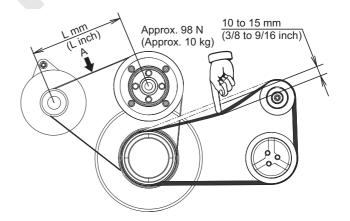
Checking method of tension
