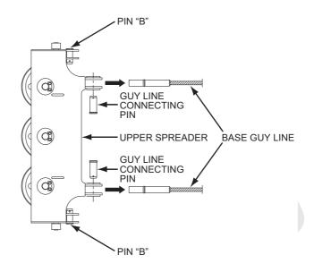
(3) Operate the boom hoist control lever to tighten the boom hoist wire rope to remove load from the bottom connector section, then draw out the bottom connecting pins.
