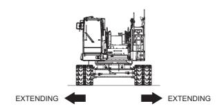
(7) If the crawler can not be extended with main machinery faces front due to ground condition, swing the upper machinery slowly to right angle with the crawler.
