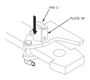
(7) Retract the crawler to the retracted position and confirm that the pin "L" is inserted. Then set the retaining pin and fix with the lock pin.
