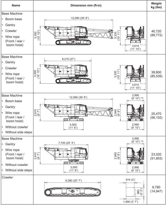
\*1 With the side step on cabin side : 3,170 (10' 5") With the side steps on the both side : 3,340 (11') In case of self-removable counterweight specifications, add 860 kg (1,896 lbs) to this weight.
