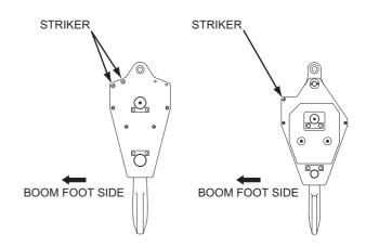
When installing the rope socket to the boom point, pay attention on the side of rope socket.
