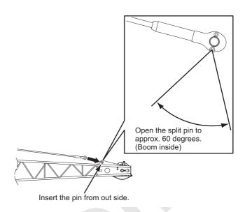
Install the jib guy line link to the boom insert with lug, referring to the "Boom and guy line configuration chart".
