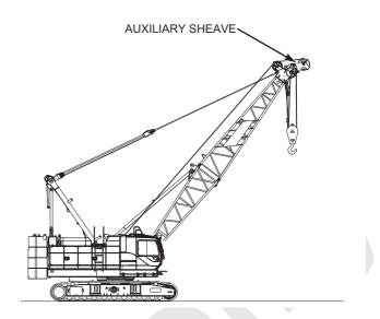
Install the auxiliary sheave installation position at the boom top, and fix it with the pin.
