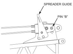
6. Wind up the boom hoist rope to the boom hoist drum paying attention not making rough spooling.
