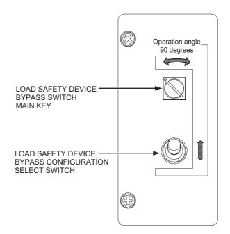
LOAD SAFETY DEVICE BYPASS SWITCH MAIN KEY
