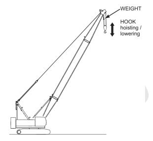
(2) When the boom is raised to approx. 82 degrees of boom angle, boom raising must be auto-stopped.
