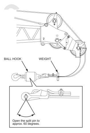
5. CONNECTING THE LOAD SAFETY DEVICE
