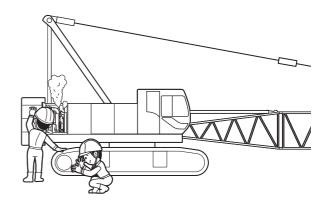
24. Pressure in hydraulic systems can be retained for long periods of time. If not properly released before maintenance people attempt to work on the hydraulic systems, this pressure can let machinery move or cause hot oil and hose ends to shoot out at high speed.
