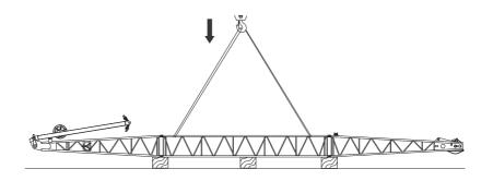
6. Remove the connecting pins between the strut and the jib tip and the connecting pins between the jib base and jib insert.
