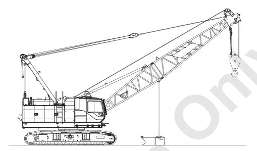
8. Remove No.2 carbody weight from the carbody in the same way as No.1 carbody weight.
