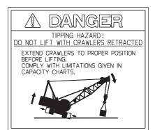
If machine swings or is assembled / disassembled with crawler retracted, main machinery may turn over to rear side.
