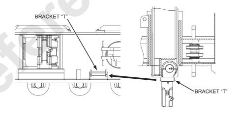
(10) Rotate all four axle extensions for 90 degrees toward inside to make them right angle with axles.
