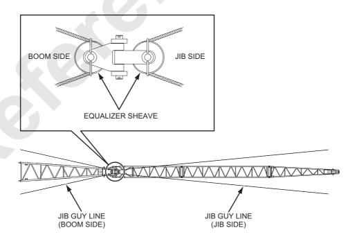
5. Connect both end of the jib guy line to the top end of the jib.
