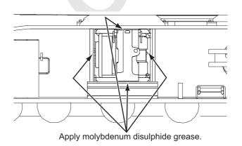
(2) Take out the clearance adjusting shims between the crawler and the axle. Stow the removed shims as shown in the figure.
