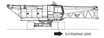
(8) Check to see that there is no obstacles in the crawler extending side. Turn the crawler ext/ret control switch to [EXT] side to extend the crawler. If the crawler can not be extended smoothly, repeat extending and retracting motions or propel forward or backward of the extending side crawler slightly while extending.
