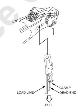
5. When installing the rope socket to the boom, insert the mounting bolt from the boom inner side and fix it with the nut and split pin from outer side.
