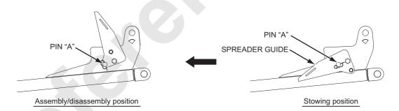
(2) By following the procedure (B) in "HOW TO USE SPREADER GUIDE" connect the spreader and the boom base bracket with the pin "B". Then remove the guy line connecting pin and remove the base guy line from the upper spreader.
