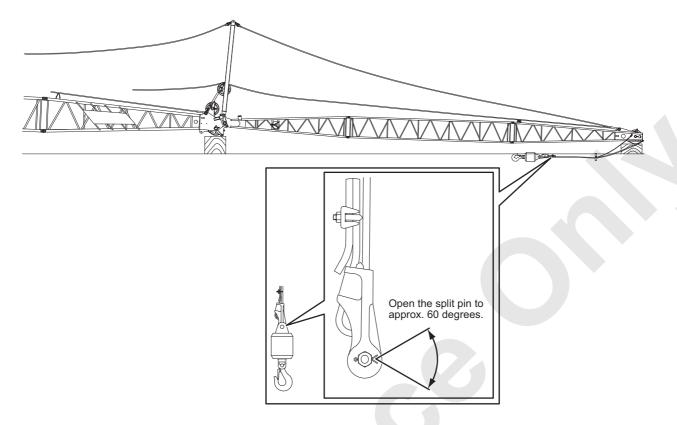
Referring to chapter "3. LOAD SAFETY DEVICE", connect the wiring for the auxiliary hoist hook antitwo block (overhoist) limit switch.
