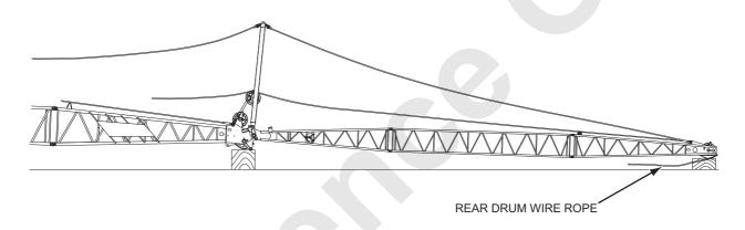
3. Install the hook overhoist limit switch and weight to the jib point section.
