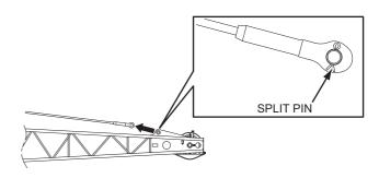
4. Take off the strut equalizer sheave and jib guy line. Re-install the removed equalizer sheave back to the original position.
