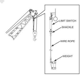
4. Pass the front drum wire rope through the hook sheave(s) and boom point sheave(s) in order. Do no forget to pass the wire rope through the weight for the overhoist limit switch. Fix the wire rope end to the boom point for even number part reeving and to the hook for odd number part reeving with the rope socket.
