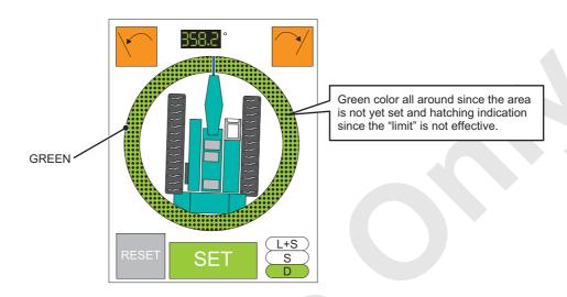
(B) Swing the crane to the place just before the obstacle on the left side and stop and push the icon [LEFT LIMIT POSITION SET].
