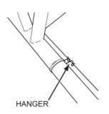
(B) Connection of attachment harness and main machine harness
