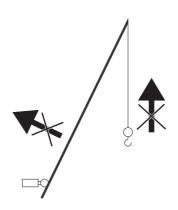
Normally when boom overhoist occurs, controller functions to stop automatically. If auto-stop function is being released and operated, the final stop limit switch control becomes actuated and machine auto-stops.
