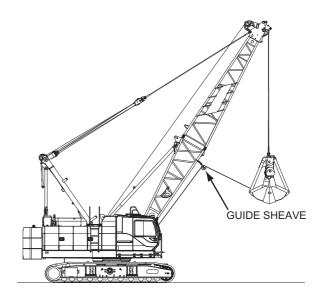
7. Adjust the wire rope tension with the tagline adjusting knob. Be sure to turn it carefully.
