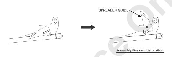
2. Use the spreader guide, and install the upper spreader on the boom base with the pin "B".
