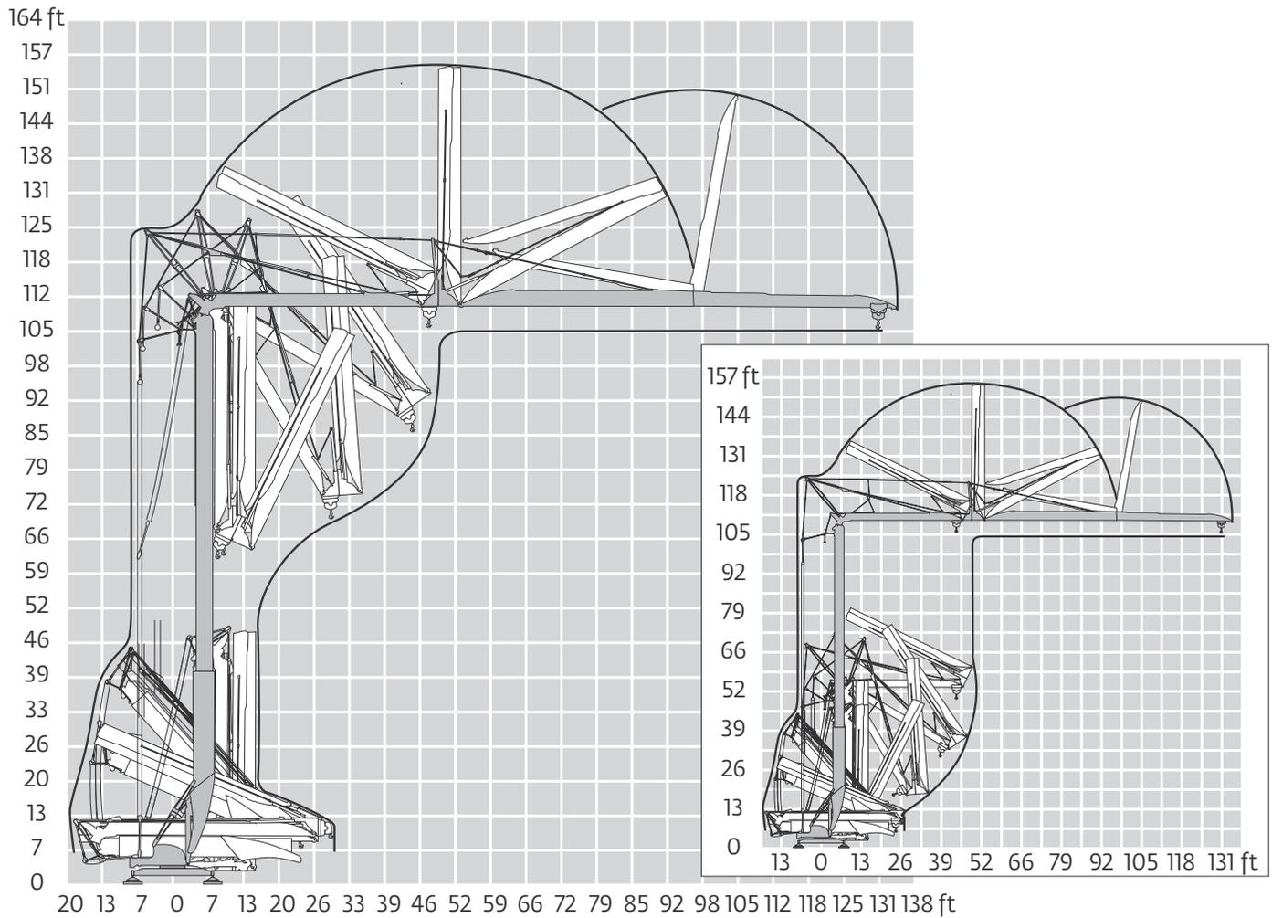
*There are two possible profiles for the Igo T 70 that are beneficial for erecting and dismantling on congested job sites.*
