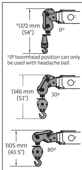
Dimensions are with the boom horizontal and the anti-two block bottomed.
