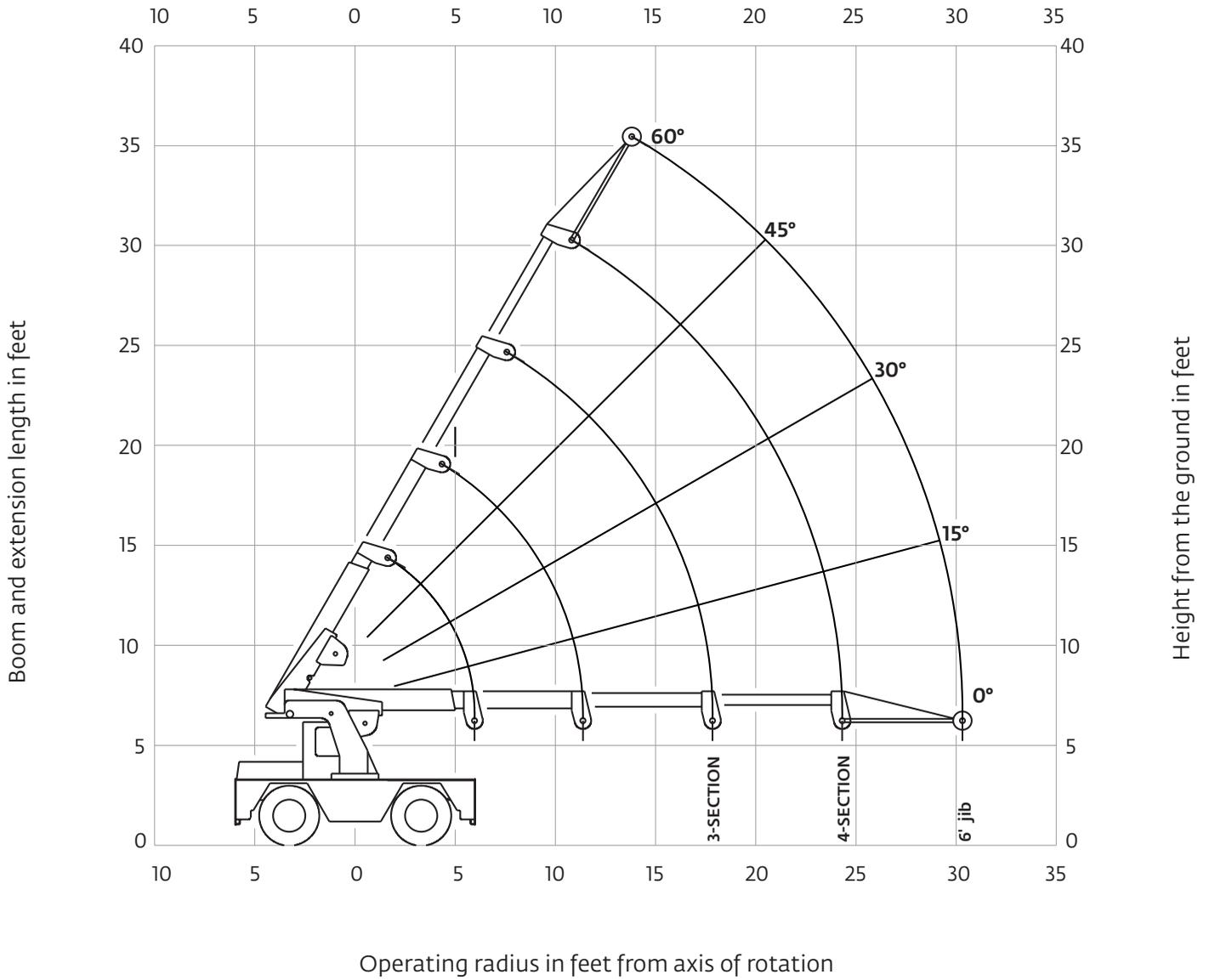
THIS CHART IS ONLY A GUIDE AND SHOULD NOT BE USED TO OPERATE THE CRANE.
