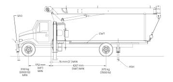
Requires front SFO stabilizer to give machine full capacity 360° around the truck. Truck must meet the minimum requirements above. Front stabilizer gives the machine a solid base, helping the operator control loads precisely.
