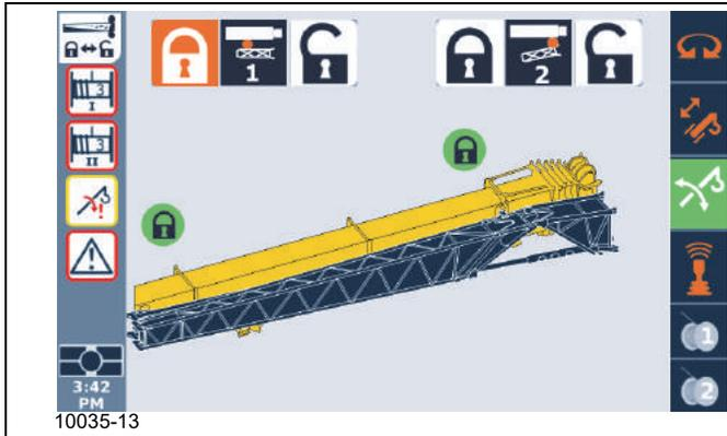
15. Visually confirm that the front boom extension pin (Pin #2 in the ODM) is locked. The handle should be in the up position. When the handle is in the up position, the front mounting pin is extended and the boom installation pins are unlocked. Lock the handle (1, Figure 5-39) with pin (2).
