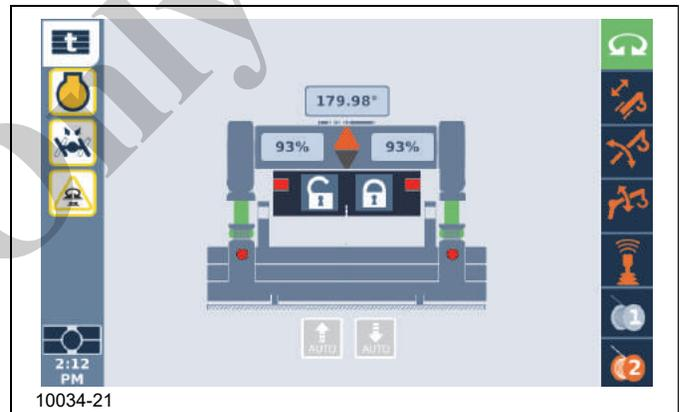
13. Using the ODM navigation control pad or jog dial, highlight the lock icon
