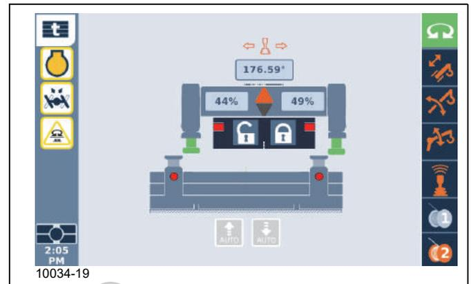
When the counterweight cylinders are fully retracted, the counterweight is removed.
