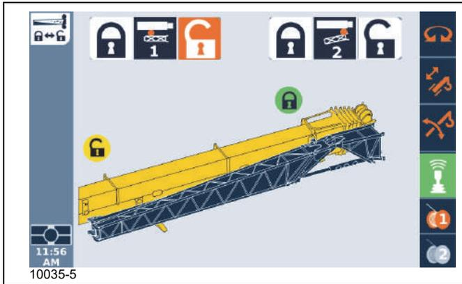
12. Visually confirm that the rear mounting pin (Pin #1 in the ODM) is unlocked.
