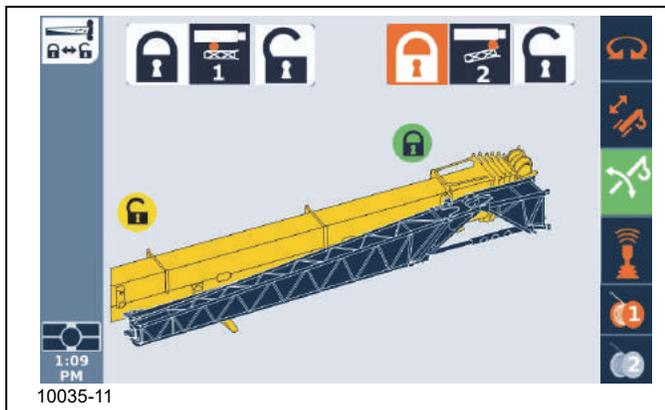
16. Make sure the ODM shows that the front mounting pin (Pin #2) is extended. Visually confirm that the front mounting pin is securely installed. Lock the handle (1, Figure 5-39) with pin (2).
