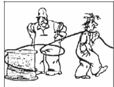
Under no circumstances, however, is the wire rope to be pulled sideways from the coil or reel, because torsion is introduced into the wire rope for each turn pulled off. Each twisting of the rope changes the lay lengths of strands and wire rope and thus also the length ratios of the rope elements in relation to each other and ultimately the load distributions in the rope.
