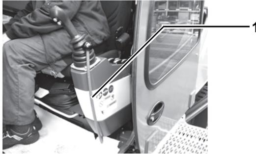
Fig. 68 Safety lever activated (pulled back)
