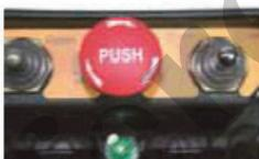
Unlock stop button by turning clockwise
