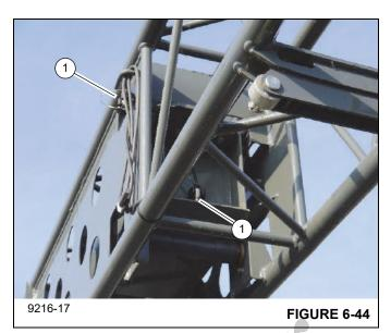
Remove the pin (1), (Figure 6-45) securing the telescoping section to the base section.
