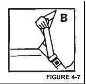
To reduce slack in the belt, pull the belt out as you did in Step 4.a.
