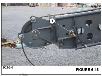
5. Connect the boom extension stinger section anti-two block cable end connector to the anti-two block switch at the nose of the boom extension stinger section. Stow A2B cable.
