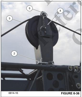
Reeve the hoist rope (3), (Figure 6-36) over the mast sheave by removing the retaining pin (5), (Figure 6-36), and routing the hoist rope over the mast sheave. Reinstall the hoist rope retaining pin (5), (Figure 6-36)
