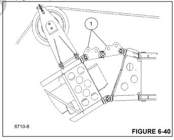
Slowly elevate and telescope the boom at the same time until the offset brackets (1),(Figure 6-40) are fully extended. **5.** Raise the boom until the offset pin takes the full load of the swingaway.
