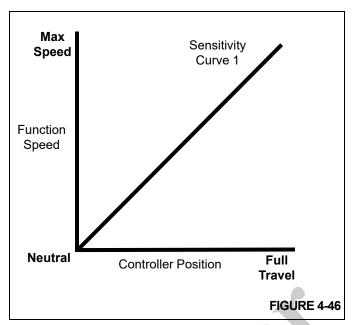
Selecting a sensitivity curve of 2 through 5 causes the function speed to be reduced, from the default sensitivity curve 1, relative to the same controller position over the full travel of the controller (Figure 4-47). Sensitivity curve 1 (default) is the most sensitive and sensitivity curve 5 is the least sensitive (Figure 4-47).
