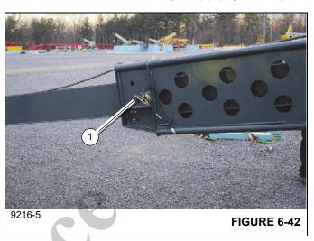
**8.** Unwind the A2B cable from the side of the boom extension base section before pulling the stinger out.
