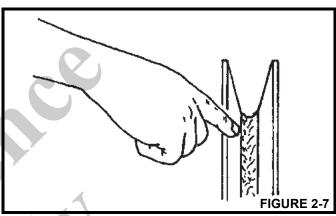
Inspect the boom nose and hook block sheaves for proper operation, excessive wear, and damage every 50 hours or weekly. Inoperable, damaged and/or worn sheaves cause rapid deterioration of rope.
