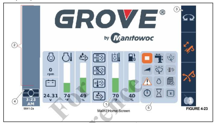
The Main (Home) Screen (Figure 4-23) appears on the ODM (lower display) when the key switch is initially set to the ON position.
