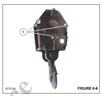
Positioning/Removing the Hoist Cable
