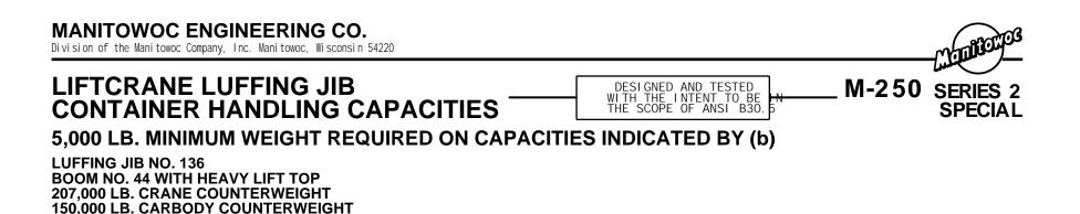
CAPACITIES FOR BOOM AND LUFFING JIB LENGTH, VARIOUS BOOM ANGLES AND LUFFING JIB OPERATING RADII ARE FOR FREELY SUSPENDED LOADS AND DO NOT EXCEED 75% OF A STATIC TIPPING LOAD. CAPACITIES BASED ON STRUCTURAL COMPETENCE ARE DENOTED BY AN ASTERISK (\*). CAPACITIES INDICATED BY (b) REQUIRE 5,000 LB. MINIMUM WEIGHT (BLOCK PLUS LOAD RIGGING) SUSPENDED FROM LUFFING JIB.
