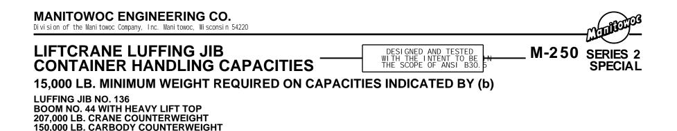
CAPACITIES FOR BOOM AND LUFFING JIB LENGTH, VARIOUS BOOM ANGLES AND LUFFING JIB OPERATING RADII ARE FOR FREELY SUSPENDED LOADS AND DO NOT EXCEED 75% OF A STATIC TIPPING LOAD. CAPACITIES BASED ON STRUCTURAL COMPETENCE ARE DENOTED BY AN ASTERISK (\*). CAPACITIES INDICATED BY (b) REQUIRE 15,000 LB. MINIMUM WEIGHT (BLOCK PLUS LOAD RIGGING) SUSPENDED FROM LUFFING JIB.
