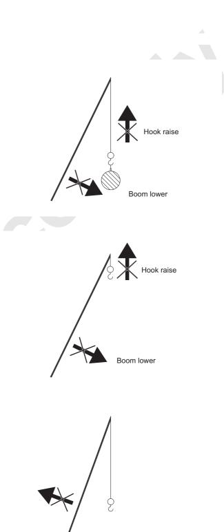
(4) Boom overhoist (Final stop limit switch control)
