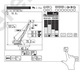
The crane turns to the simulated overload condition and auto-stop occurs. (Overload check mode)
