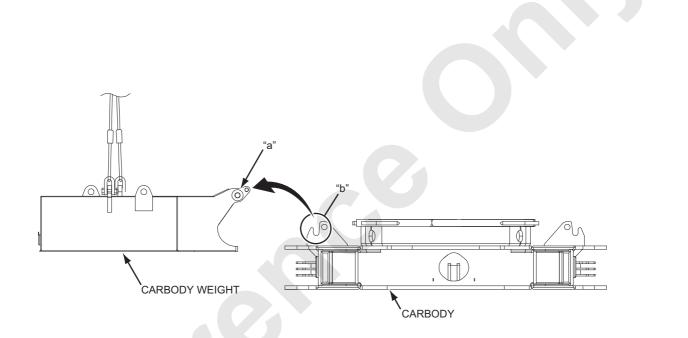
4. Remove No.2 carbody weight from the carbody in the same way as No.1 carbody weight.
