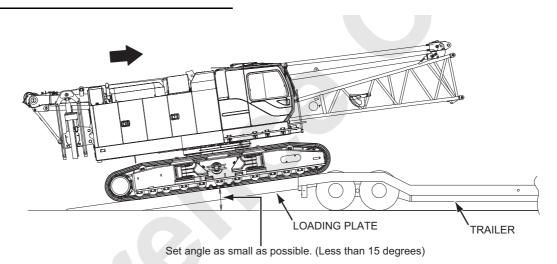
(3) Secure the lower machinery to the trailer with the wire rope or chain to prevent it from cargo collapsing.
