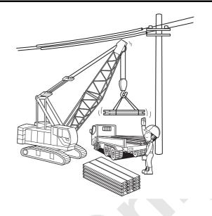
3. If coming close to the power line is unavoidable, advise the power company and obtain the protective insulated tube to prevent electric shock.
