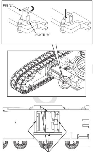
Apply molybdenum disulphide grease.
