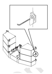
7. Propel the crane to the position where the counterweight link and the base machine counterweight link can be connected.
