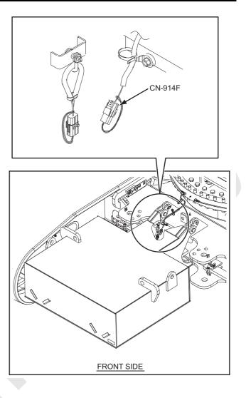
5. Lift up No.1 carbody weight using the boom base and disconnect "a" area of carbody weight from "b" area of the carbody.
