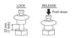
These knobs are to lock the drum to for safety during lowering the lifting load or boom.
