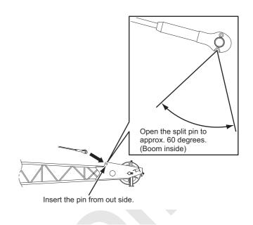
6. Install the jib guy line link to the boom insert with lug, referring to the "Boom and guy line configuration chart".
