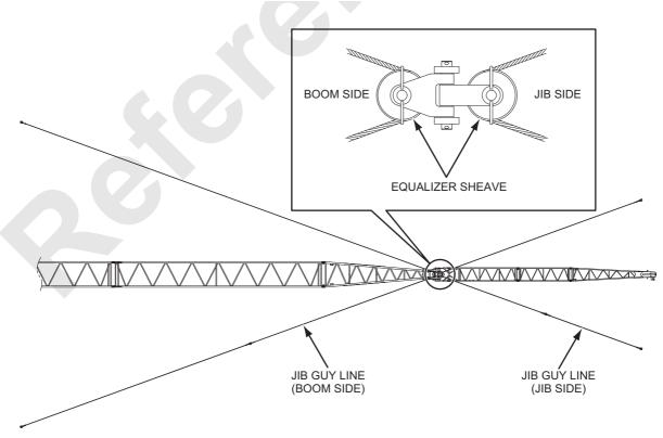
5. Connect both ends of the jib guy line to the top end of the jib.
