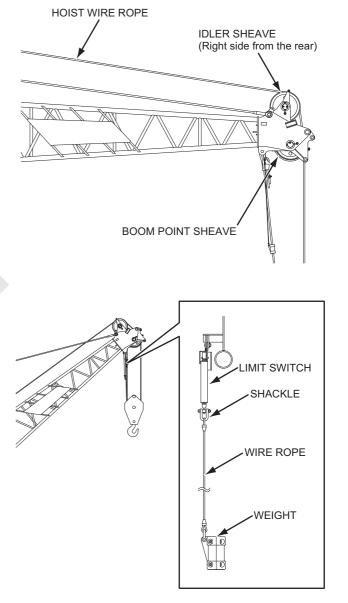
Pass the front drum wire rope through the hook (s) and boom point sheave (s) in order.
