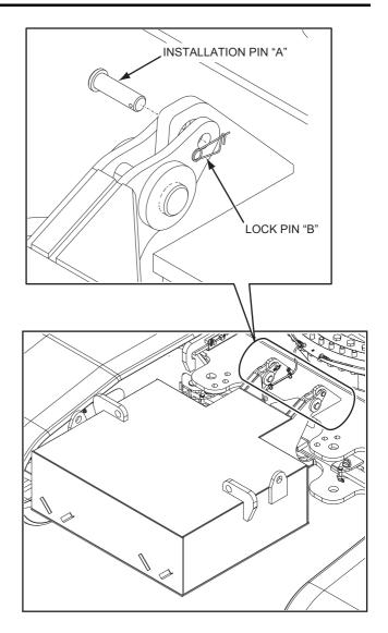
(14) Installing No.2 WEIGHT Install No.2 WEIGHT in the same way as No.1 WEIGHT.
