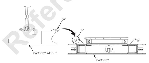
(13) Insert the carbody weight installation pin "A" and secure it with the lock pin "B".
