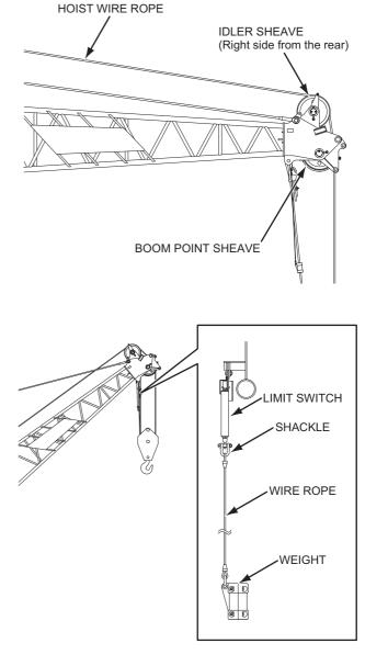
4. Pass the front drum wire rope through the hook sheave(s) and boom point sheave(s) in order. Do no forget to pass the wire rope through the weight for the overhoist limit switch. Fix the wire rope end to the boom point for even number part reeving and to the hook for odd number part reeving with the rope socket.
