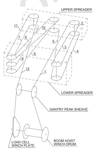
(3) Fix the wire rope end to the winch bracket using the socket, wedge and clamp.
