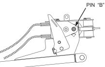
(C) When stowing the spreader guide, slowly tighten the boom hoist wire rope. When there becomes clearance between the spreader and the spreader guide, draw out pin "A", and return the spreader guide to the stowing position.
