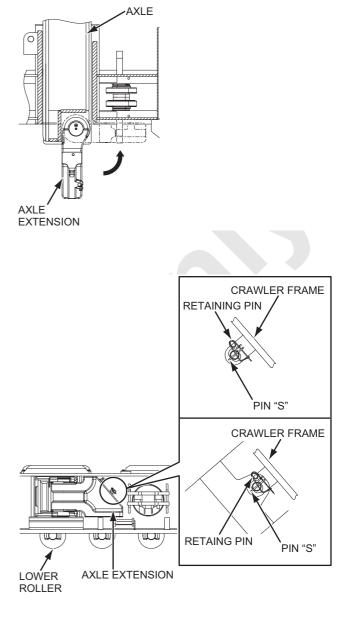
(11) Secure the axle extension and crawler frame with the pin "S" and insert the retaining pin.
