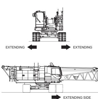
(7) If the crawler can not be extended with main machinery faces front due to ground condition, swing the upper machinery slowly to right angle with the crawler.
