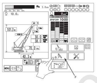
(3) Work area limit setting screen becomes indicated.(The screen example is crane case.)Push the figure area if new setting is required.
