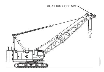
Install the auxiliary sheave installation position at the boom top, and fix it with the pin.
