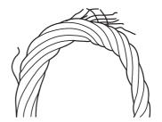
Bend rope sharply to expose breakage.
