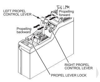
Propel speed is regulated by turning the accelerator grip, and by proportionally pushing and pulling the propel control levers.
