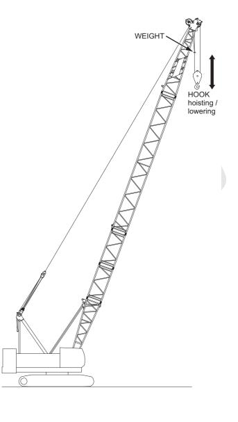
(2) When the boom is raised to approx. 82 degrees of boom angle, boom raising must be auto-stopped.
