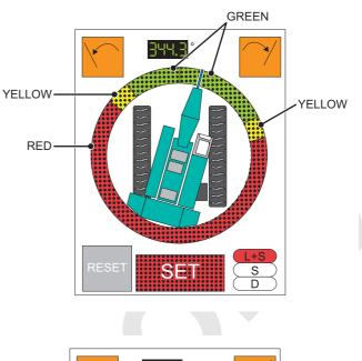
(B) To set again, push [RESET] icon. The screen returns to the one shown right. Set again based on new setting procedure (P.3-54).
