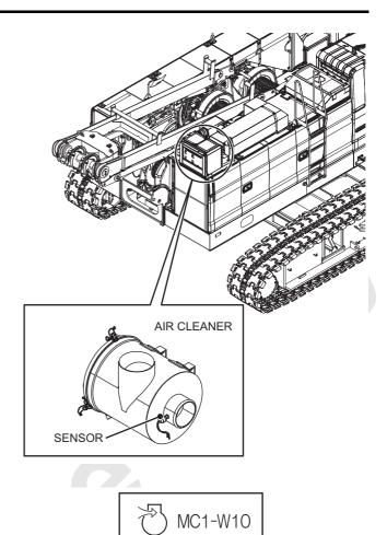
The engine air cleaner is clogged. Clean or replace the element.
