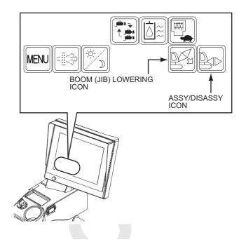
5. By lowering the boom further, the hook overhoist limit switch operates when the weight of the hook overhoist limit switch is placed on the ground, and the boom lowering is automatically stopped again. Press and hold the "Assy/disassy" icon one time for approx. 1 second and it becomes the Assy/disassy mode, and the boom can be lowered. Be careful because the hook overhoist automatic stop does not function in the Assy/disassy mode.
