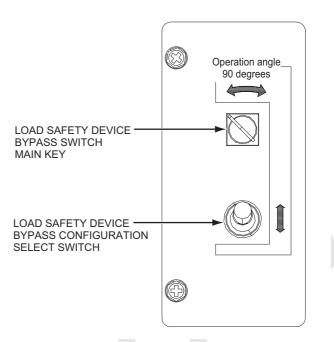
LOAD SAFETY DEVICE BYPASS SWITCH MAIN KEY
