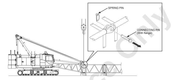
3. DISASSEMBLING THE BOOM INSERT Disconnect the boom insert in order by removing the connecting pins.
