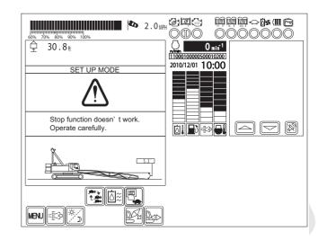
STOP RELEASE MODE WHEN TRANSPORTA-TION WITH BOOM BASE ATTACHED.
