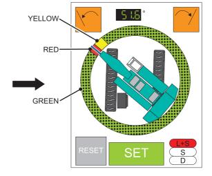
(C) Swing the crane to the place just before the obstacle on the right side and stop and push the icon [RIGHT LIMIT POSITION SET].The crane figure swings to right. Push [RIGHT LIM-IT POSITION SET] icon after stop.
