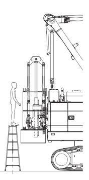
6. Pull out the weight support pin using an extension bar.
