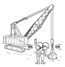
21. If there is not enough wire rope on the drum the rope can snap loose.
