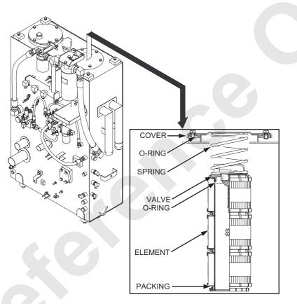
(1) Remove the filter assembly and place it on the flat surface.
