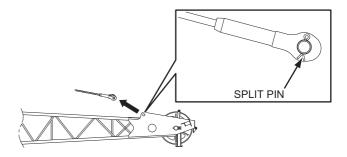
4. Take off the strut equalizer sheave and jib guy line. Re-install the removed equalizer sheave back to the original position.
