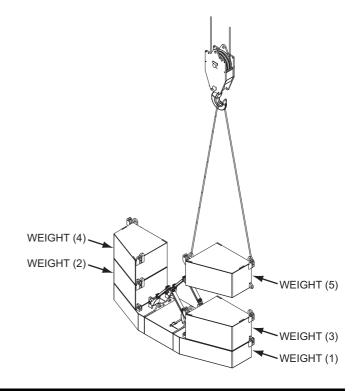
6. Secure right and left counterweights with the connecting pins respectively and retain them with the spring pins. (8 locations)
