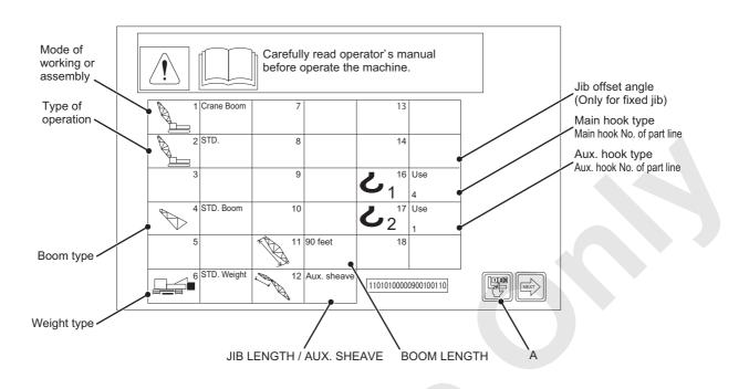
Then setting condition of work area limit becomes indicated. After checking the content, push [OK] icon.
