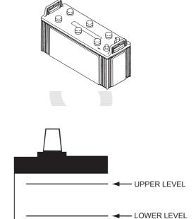
(2) When you cannot check the battery electrolyte level from the side level line, or no level lines are provided on the side of the battery:
