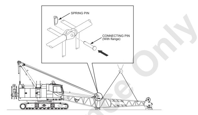
2. Raise the boom base until the lower pin holes are aligned with each other. Then tap the connecting pins (double tapered pin) in, and insert the spring pins into the both ends of the connecting pin.
