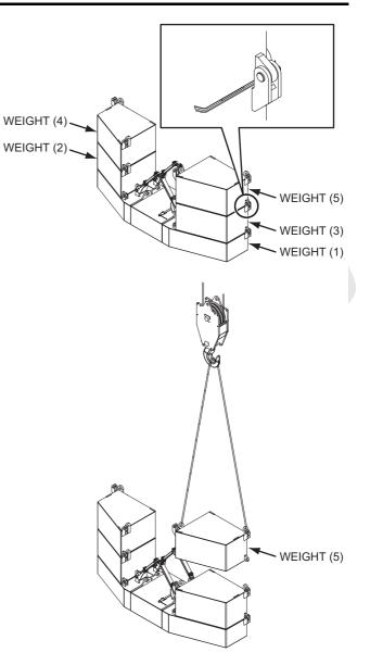
3. Lower the links by removing the pin and lock pin.
