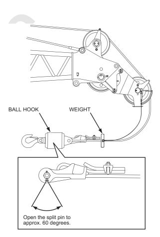
5. CONNECTING THE LOAD SAFETY DEVICE
