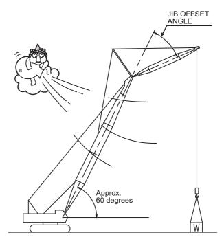
In case when the wind speed is expected to exceed 67 MPH.
