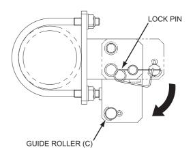
3. Take out the roller of the guide roller (C) to the work positions and secure with the lock pin.
