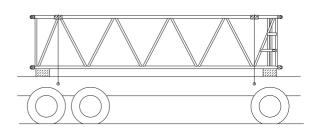
When placing a boom upon another boom, place blocking just above the under blocking.
