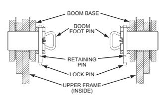
4. Hold the boom base foot area with the assisting crane and pull out the cab side (right hand) boom foot pin first and then left side boom foot pin.
