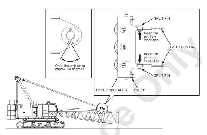
5. Use the spreader guide to remove the pin "B".
