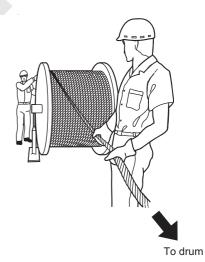
Kink: Deformation by twisting of wire rope
