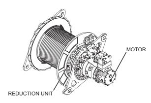
FRONT, REAR DRUM MOTOR AND REDUCTION UNIT
