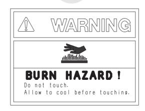
During engine running or straight after the engine is stopped, inside of the radiator becomes high pressure and hot.
