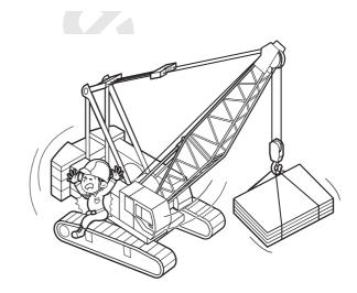
5. People can be crushed by the rear (counterweight) of the machine if there is not enough room for it to swing.
