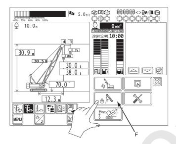
(3) Work area limit setting screen become indicated. (The screen example is crane case.)
