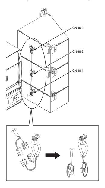
2. Connect the remote control cable to the receptacle located under the right deck.
