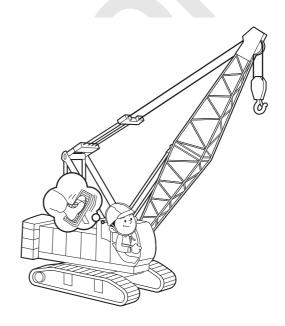
23. Trying to repair or adjust equipment with a suspended hook or load or with the boom raised could release machinery and let it move unexpectedly. Always lower the load to the ground and the boom onto proper cribbing before doing maintenance or repair work.
