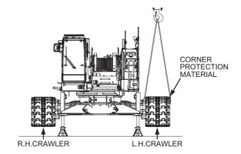
(3) While the crawler is being held, extend the left side crawler toward outer side by controlling the left crawler extend control switch of the remote controller
