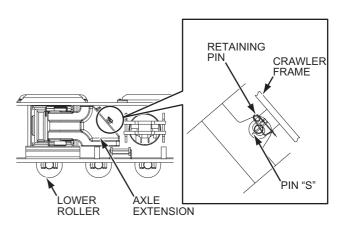
(3) Turn all four axle extensions for 90 degrees toward outside to make them parallel to the axles. Insert the pin "S" into the crawler frame bracket hole and secure it with the retaining pin.
