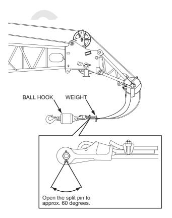
5. CONNECTING THE LOAD SAFETY DEVICE
