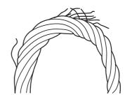
Bend rope sharply to expose breakage.
