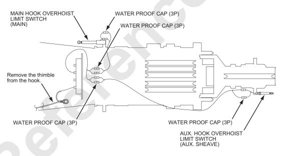
Aux. sheave installed boom tip area
