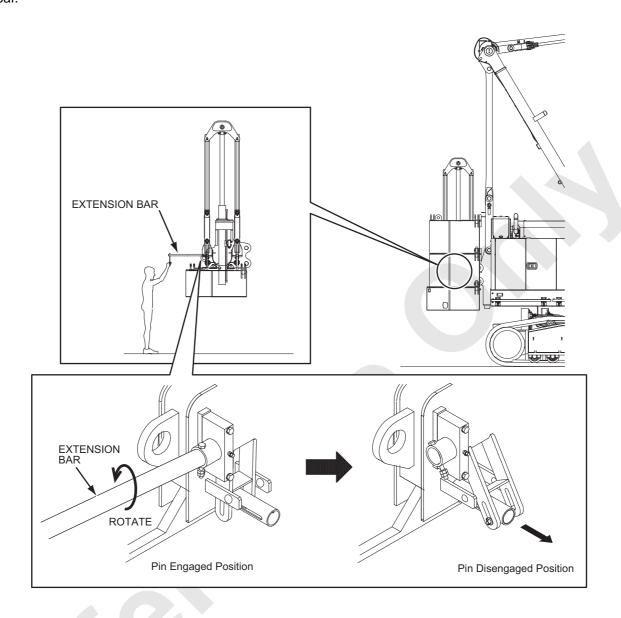
Operate the remote control to lower the counterweight until the counterweight is placed on the ground.
