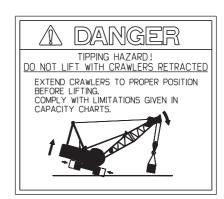
4. If machine swings or is assembled / disassembled with crawler retracted, main machinery may turn over to rear side.
