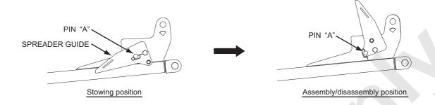
(B) Lower the boom. After the tip end of the boom has been grounded, slowly loosen the boom hoist wire rope more. The spreader is lowered along the spreader guide. When the hole of the spreader is aligned with the pin hole of the bracket on the boom base section, insert pin "B" to connect the spreader to the base boom bracket.
