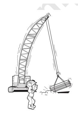
20. Trying to lift a load which is stuck, frozen or attached to something else may result in tipping, boom collapse or other damage.
