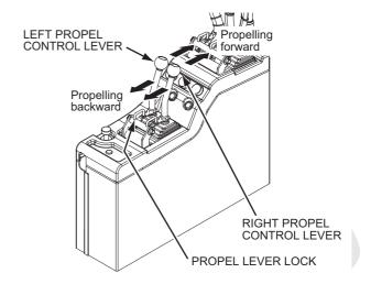
Propel speed is regulated by turning the accelerator grip, and by proportionally pushing and pulling the propel control levers.
