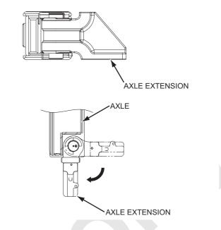
(3) Extend the axle extension and then set the bracket "T" as shown.
