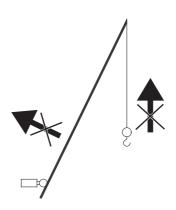
Normally when boom overhoist occurs, controller functions to stop automatically. If auto-stop function is being released and operated, the final stop limit switch control becomes actuated and machine auto-stops. In this case, auto-stop can not be released.
