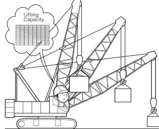
2. Cranes may tip over or collapse if the operating surface cannot support their weight.
