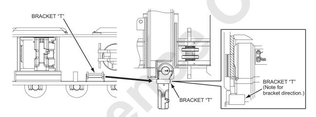
(5) Take out the clearance adjusting shims between the crawler and the axle.
