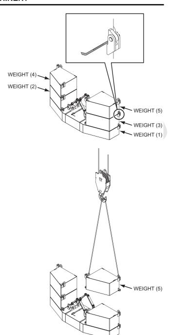
3. Lower the links by removing the pin and lock pin.
