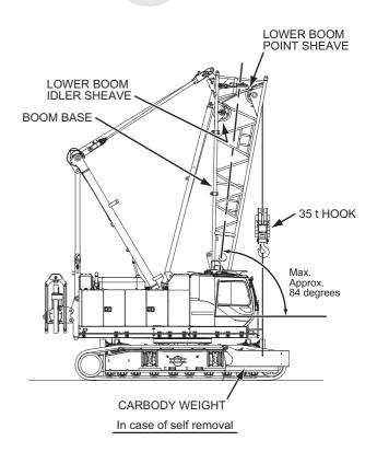
(B) Install the "a" area of the carbody weight to the "b" area of the carbody.
