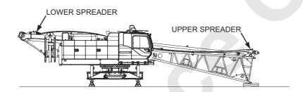
(2) Remove the wire rope from the boom hoist winch link.
