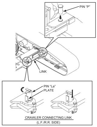
(12) While holding the crawler with the lower boom, extend the crawler to the work position by extending the cylinder and check that the pin "La" and "Lb" which has been placed on the link is inserted into the link hole.
