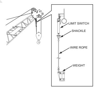
4. Pass the front drum wire rope through the hook (s) and boom point sheave (s) in order.
