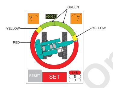
(5) After swing motion stops, swing left to returns the crane to safe area (green area immediately.
