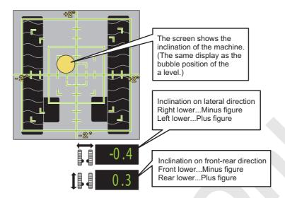
The above figure indicates example of condition that right rear part is lower.
