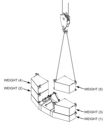
5. Secure right and left counterweights with the connecting pins respectively and retain them with the spring pins. (8 locations)
