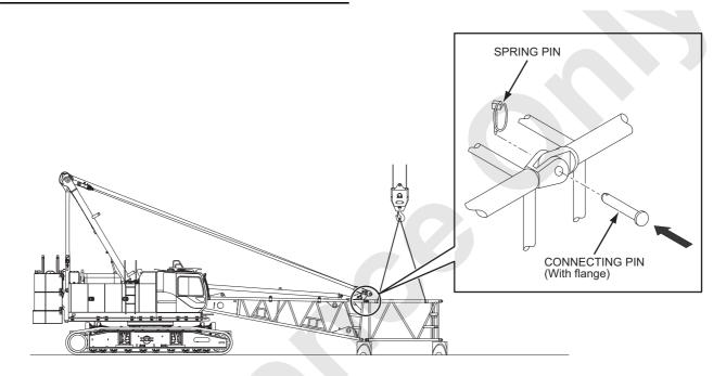
(3) Lift up the connecting section of the boom base and the boom insert and align the bottom connecting pin holes, and insert the connecting pins (double tapered pin) into these holes. Insert the spring pins into the connecting pins to fix them.
