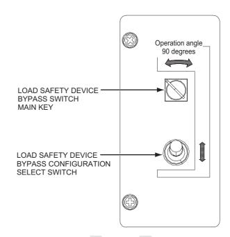
LOAD SAFETY DEVICE BYPASS SWITCH MAIN KEY
