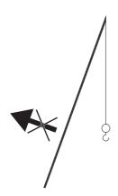
(4) Boom overhoist (Final stop limit switch control)
