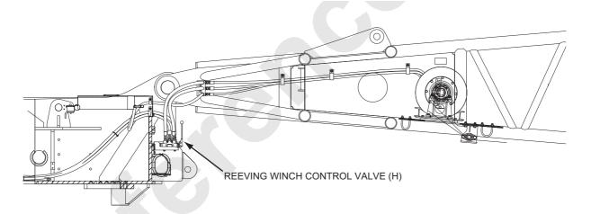
4. Connect the hoses from the reeving winch control valve (H) to the piping block (J) on the boom base left side with each hose coupler (E) (F) (G). Connect each hose coupler so that the male and female fitting of the piping block (J) matches each other.
