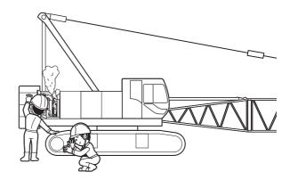
24. Pressure in hydraulic systems can be retained for long periods of time. If not properly released before maintenance people attempt to work on the hydraulic systems, this pressure can let machinery move or cause hot oil and hose ends to shoot out at high speed.
