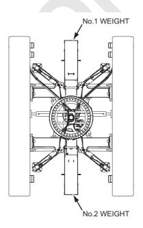
There are two way to install the carbody weight.
