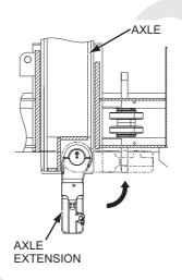
(11) Secure the axle extension and crawler frame with the pin "S" and insert the retaining pin.
