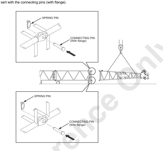
As an alternative way of attachment connection, the boom inserts and boom top are to be connected first and then the boom base and the boom inserts can be connected as last as shown below.
