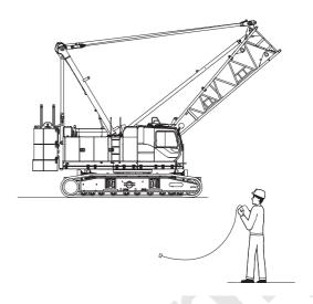
(10) If the counterweight quantity detect unit is equipped, connect the detect harnesses installed on all of the counterweights and the main machinery harness.
