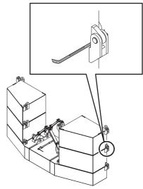
6. Move the crane to the position where the counterweight can be removed.
