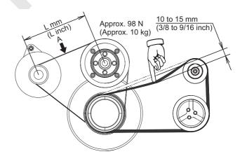
Checking method of tension
