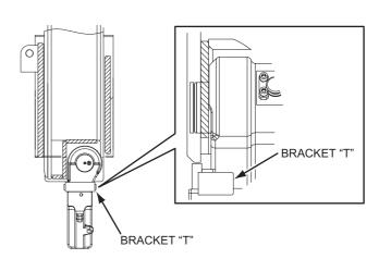
4. Rotate all four axle extensions for 90 degrees toward inside to make them right angle with axles.
