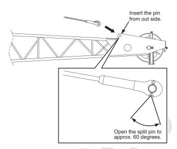
Install the jib guy line link to the boom insert with lug, referring to the "Boom and guy line configuration chart".
