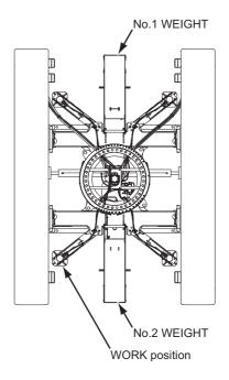
There are two way to removal the carbody weight. One is to use an assisting crane and the other is to use the machine boom base.
