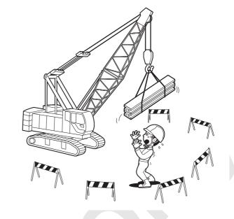
10. Rapid swings or sudden starts and stops can cause the hook and attached load to swing out of control. Always start and stop movements smoothly and swing at speeds that will keep the load under control.
