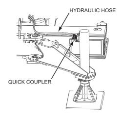
(3) Remove the pin "C" as shown right and remove the float from the vertical cylinder.
