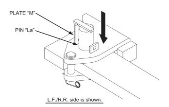
(10) By extending the crawler to the extended position, the pin "La" and "Lb" will be inserted into the pin hole.
