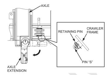
(4) Insert the axle extension retaining bracket "T" to the foot area of the axle extension from the direction as shown lower.
