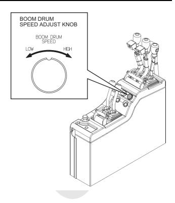
When the boom approaches the upper limit angle, the hoisting speed is reduced. The angle to start the speed reduction differs depending on the engine speed.
