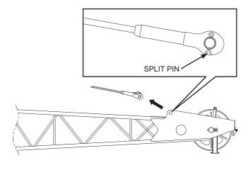
4. Take off the strut equalizer sheave and jib guy line. Re-install the removed equalizer sheave back to the original position.
