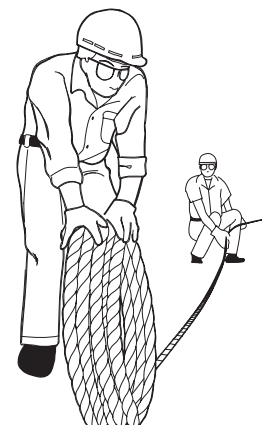
Unreeving method of wire rope
