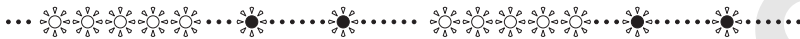
(The pattern after blinking short plus signal 5 times, long plus signal 2 times and repeat.)
