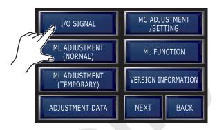
How to select the in/out signal display Select the controller to confirm signals and select signal so the each input/output signal screen is to be displayed.
