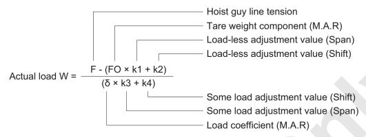
Suppose the values above are indicated shown below and the indicated actual load is 2 t, when a load weighing 5 t is lifted with the front winch.
