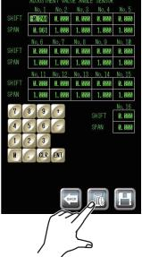
(7) All adjustment data returns to the initial value. Initial value: Shift = 0.000, Span = 1.000
