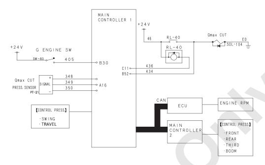
(1) G engine function select switch After inputting into select switch, check the each levers location and if they are all in neutral, Q max cut solenoid is energized.
