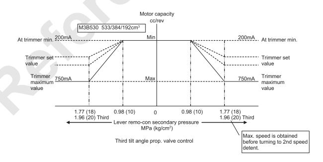
(B) Maximum current of motor tilt angle prop. valve is controlled by no load engine speed (Command quantity by grip).
