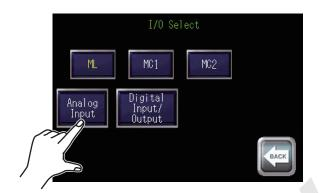
(2) Unit of indicating figure is V (volt). Refer to the article "10.2.4 DETAIL OF ML CONTROLLER" for connection and signal level. 0V is displayed on non connected point.
