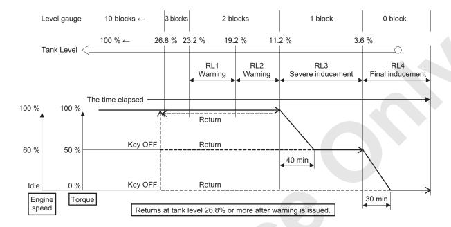
DEF/AdBlue<sup>®</sup> tank level lower (The method of release when display RL1 or RL2 on the monitor)
