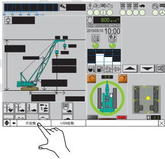
If the error as shown right is displayed, check for inserted condition of CF card or cover to be closed.
