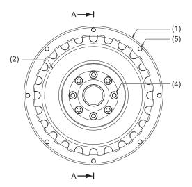
Tightening torque: 71.1 to 86.9 N·m (52.4 to 64.1 ft·lbs)
