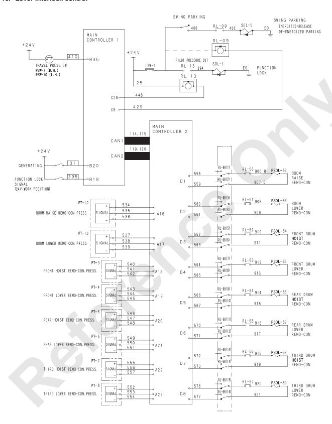
This is to prevent drum unexpected rotation at engine start when the lever is in operating position and the function lock lever is in work position.
