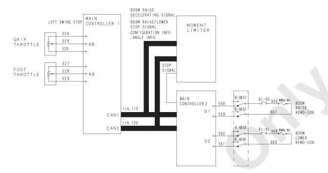
When boom raise deceleration signals are input (input when the boom reaches 10 degrees before the boom upper limit), the boom raise remote control proportional valve is controlled and the boom raising speed is decelerated according to the boom angle.
