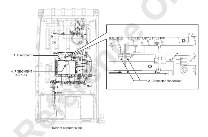
During download, 7 segment display of the controller changes as shown below.
