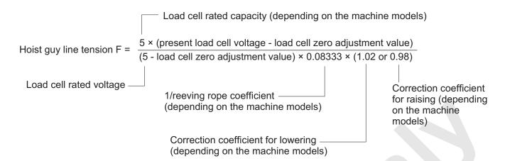
If the load cell zero point adjustment has not been carried out, adjustment value is 1, and the coefficient is 1.02 if the boom lowering stopped.
