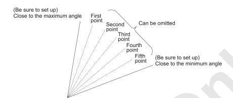
Max. boom (jib) angle and min. boom (jib) angle points are essentially required but points between them can be neglected.
