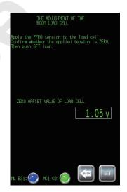
(3) The message shown right becomes indicated when the adjustment is properly completed. By pressing [SET], screen returns to the previous one.
