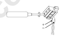
(4) Handling of the bypass switch when touch panel of the monitor dose not functioning
