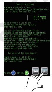
(8) If the adjustment is properly completed, the message shown right is displayed.
