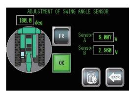
(4) When either FR or RE is pressed and "NG" is displayed, adjustment is in error.
