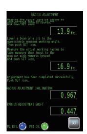
(8) If the adjustment is not properly completed, the message shown right is displayed.
