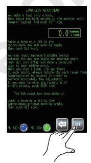
(8) If the adjustment is properly completed, the message shown right is displayed.
