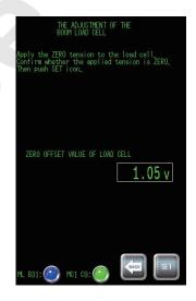
(3) The message shown right becomes indicated when the adjustment is properly completed. By pressing [SET], screen returns to the previous one.
