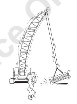
20. Trying to lift a load which is stuck, frozen or attached to something else may result in a tipping, boom collapse or other damage. Be sure that loads are free before lifting.
