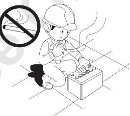
Disconnect the battery cables during inspection and maintenance of electrical system.
