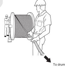
Kink: Deformation by twisting of wire rope
