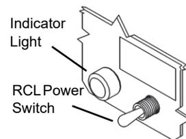
**NOTE:** The RCL power switch must be ON before the crane can be operated.
