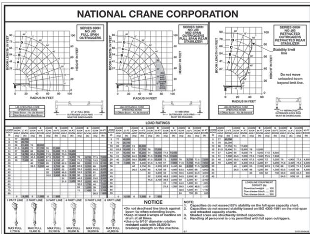
The load chart contains the lifting capacities of the crane in all allowable lifting configurations. The information is presented in three parts, one for outriggers fully retracted, one for outriggers at mid point, and one for the outriggers fully extended. Each part contains the load chart, range diagram, and hoist data sheet. In the examples shown here, the information for the outriggers fully extended is used.
