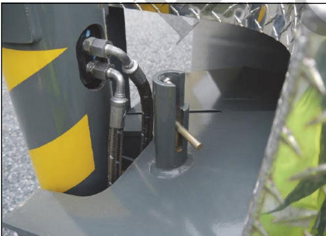
Mid-Extend Pin in Locked Position
