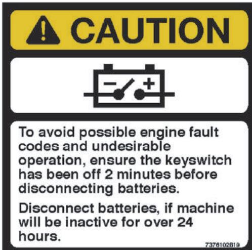
The battery disconnect switch is located on the battery box cover on the left side of the crane. To disconnect the batteries, turn battery disconnect switch to the OFF position. If necessary, lock the battery disconnect in the OFF position using a padlock. Turn switch to the ON position to connect the batteries.
