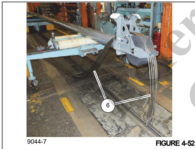
69. Remove two bolts (524) securing each wear pad (515) to left and right sides of sheave head weldment (506) (see Figure 4-53).
