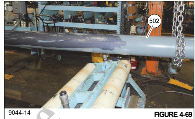
21. Using adequate chains and crane, lift telescope cylinder #1 (502) and position behind tele 3 (401) (see Figure 4-70).
