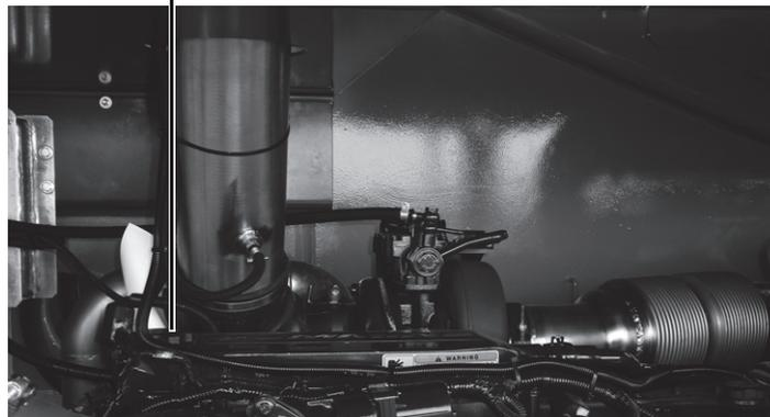
Fig. 199 Oil dipstick and oil filter neck
