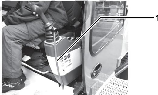
Fig. 58 Safety lever activated (pulled back)
