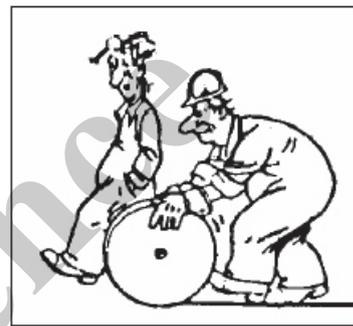
Unreeing on the ground, which is repeatedly recommended in the pertinent literature, is not very satisfactory in practice because the reel unwinds an increasingly smaller amount of rope than the distance it covers, i.e. with this approach you are forced to pull the wire rope along behind you.
