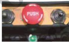
Unlock stop button by turning clockwise
