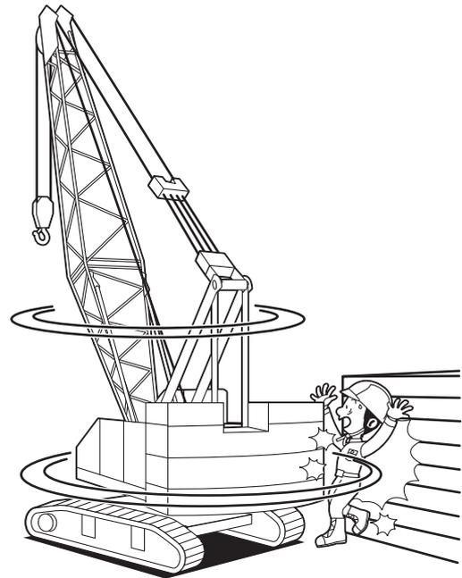
6. Many people have been injured when riding crane hooks or loads or while being lifted in man baskets. They have no control over how they are handled and no protection from impacts or falls. Small mistakes can be fatal.
