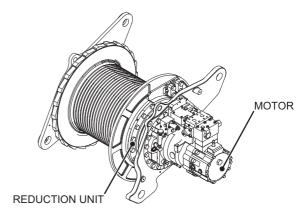
FRONT, REAR DRUM MOTOR AND REDUCTION UNIT
