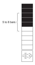
Make machine in idling condition and push the soot burning (regenerating) icon.
