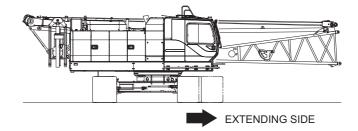
(8) Check to see that there are no obstacles in the crawler extending side. Turn the crawler ext/ret control switch to [EXT] side to extend the crawler. If the crawler cannot be extended smoothly, repeat extending and retracting motions or propel forward or backward of the extending side crawler slightly while extending.
