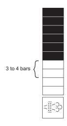
Auto regeneration becomes actuated when control lever is not used and burning (regenerating) soot start automatically.
