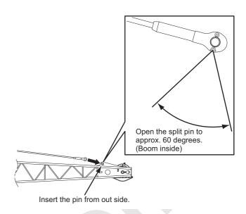
6. Install the jib guy line link to the boom insert with lug, referring to the "Boom and guy line configuration chart".
