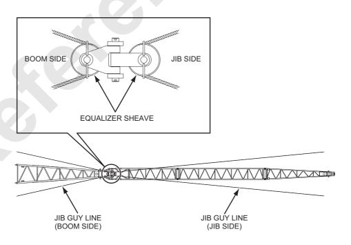
5. Connect both end of the jib guy line to the top end of the jib.
