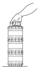
(2) Hold the top mold plate and loosen the grip.
