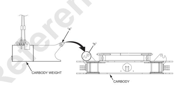
(3) Insert the carbody weight installation pin "A" and secure it with the lock pin "B".
