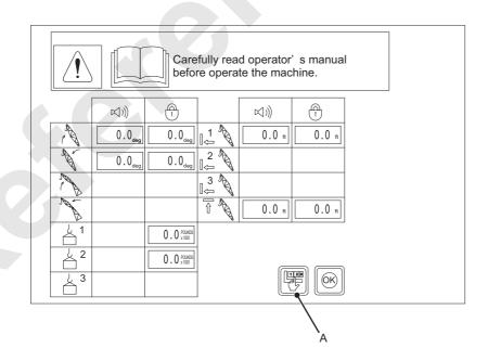
Main screen is displayed and the crane is ready to operate.
