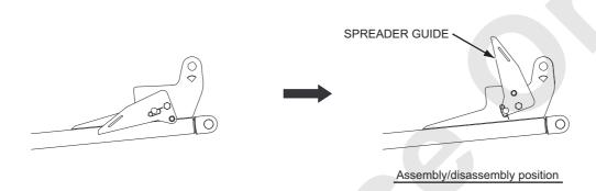
2. Use the spreader guide, and install the upper spreader on the boom base with the pin "B".
