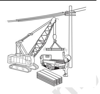
3. If coming close to the power line is unavoidable, advise the power company and obtain the protective insulated tube to prevent electric shock.
