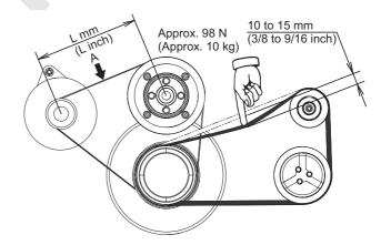
Checking method of tension
