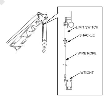
4. Pass the front drum wire rope through the hook sheave(s) and boom point sheave(s) in order. Do no forget to pass the wire rope through the weight for the overhoist limit switch. Fix the wire rope end to the boom point for even number part reeving and to the hook for odd number part reeving with the rope socket.
