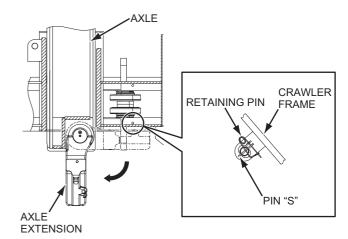
(4) Insert the axle extension retaining bracket "T" to the foot area of the axle extension from the direction as shown lower.
