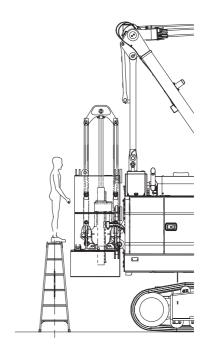
6. Pull out the weight support pin using an extension bar.
