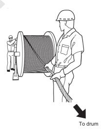
Kink: Deformation by twisting of wire rope
