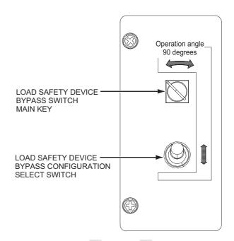
LOAD SAFETY DEVICE BYPASS SWITCH MAIN KEY
