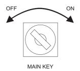
LOAD SAFETY DEVICE BYPASS CONFIGURA-TION SELECT SWITCH
