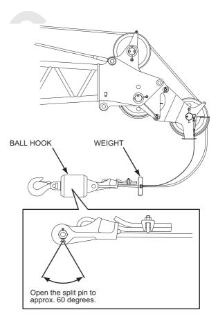
5. CONNECTING THE LOAD SAFETY DEVICE
