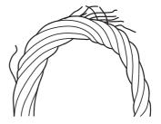
Bend rope sharply to expose breakage.
