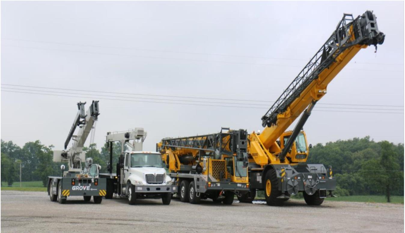
**Carry Deck / Boom Truck/Truck Mount/Rough Terrain**
