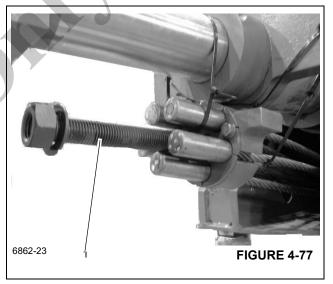
**25.** Insert the installation bolt into the inner mid anchor weldment and take up as much slack as possible.
