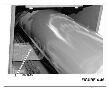
**19.** Temporarily tie extend cables to the Telescope Cylinder to maintain proper cable alignment during assembly (Figure 4-45).
