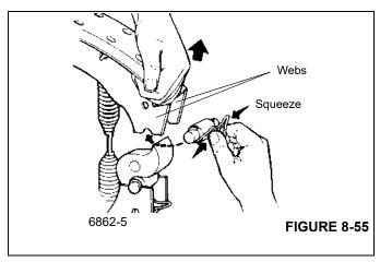
Push the retainer into the brake shoe until its ears lock into the holes in the brake shoe webs.
