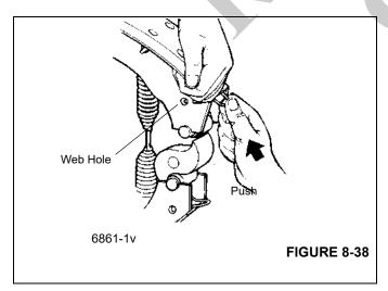
Install the slack adjuster. Reference Automatic Slack Adjuster, page 8-40.
