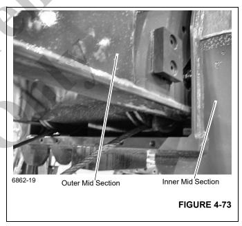
**NOTE:** Pull the mid retract cables through the base section as the sections are joined.
