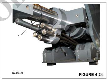
**11.** Continue to pull the assembly from the inner mid section until access to the rear of the outer mid section is gained in order to disconnect the four **retract** cables (1), (Figure 4-25).
