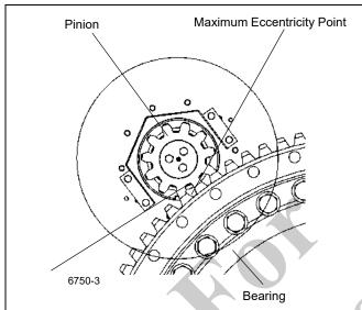
0.2 mm (0.008inch) Thick Shim By Full Width to Tooth Engagement [0.04 mm (0.016 inch) Backlash]
