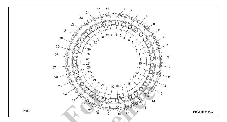
The inner race of the bearing is secured to the turntable by 36, 1 inch, grade 8 bolts. The outer race of the bearing is secured to the carrier frame by 36, 7/8 inch, grade 8 bolts.
