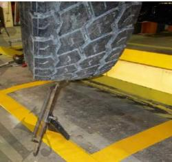
• Lower the machine to the ground. Back out and drive straight into the work area several times to ensure the vehicle's suspension components remain relaxed and achieve proper measurements. Place wheel chocks on the drive axles.
