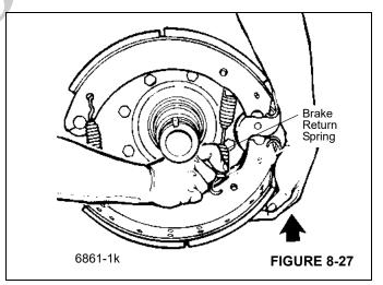
**5.** Rotate the bottom brake shoe to relieve tension on the retaining springs. Remove the springs and brake shoes.
