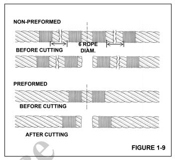
Installing 35x7Class Wire Rope
