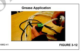
Use a clean towel (or clean glove) to remove any excess material from the surface of the connector, and wipe material into the terminal sockets as shown in (Figure 3-13)
