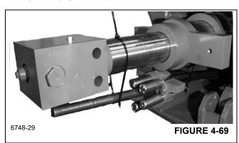
**13.** Assemble the fly retract cable anchor weldments to the retract cables. Thread the single nut on the cable end until there is 38 mm (1 1/2 inch) of thread showing, then install the locknut (Figure 4-70).
