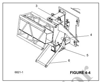
7. Extend the boom approximately 51 to 64 cm (20 to 25"). Make certain that the boom extension stowage lugs clear the guide pins (1), (Figure 4-5) and ramp (4), (Figure 4-4) on the front and rear stowage brackets.
