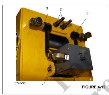
Remove the nuts and washers securing the synchronizing cable ends (2), (Figure 4-12) to the base section.
