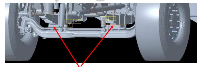
Install shims between the spring assemblies and shock plates.
