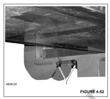
**10.** Insert the wear pads and pad holders (1), (Figure 4-53) on the left and right side of the fly section.
