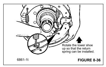
3. Pull each brake shoe away from the cam to permit enough space to install the cam rollers and retainers. Press the ears of the retainer together to permit the retainer to fit between the brake shoe webs.
