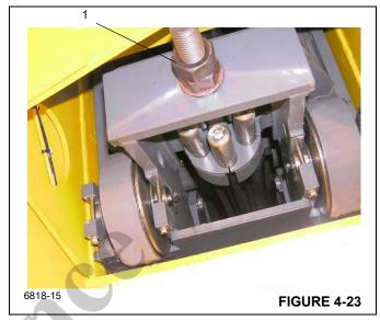
**10.** Secure the extend cable keeper plate and adjustment bolt to the tele cylinder with cable ties (1), (Figure 4-24) or tape. Failure to do so may allow the cables and keeper to become jammed during disassembly.
