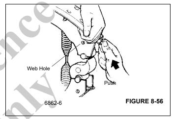
Install the slack adjuster and adjust brakes. Refer to following Sub-Section, Automatic Slack Adjuster, page 8-40.
