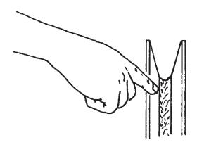
Inspect the boom nose and hook block sheaves for proper operation, excessive wear, and damage every 50 hours or weekly. Inoperable, damaged and/or worn sheaves cause rapid deterioration of rope.
