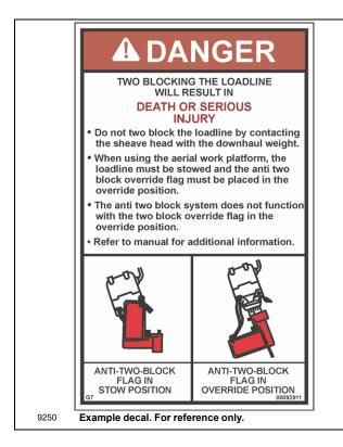
Two-blocking is more likely to occur when both the main and auxiliary hoist lines are reeved over the main boom nose and jib nose respectively. An operator, concentrating on the specific line being used, may telescope or lower the boom allowing the other hoist line attachment to contact the boom or jib nose, thus causing damage to the sheaves, or causing the rope to fail, dropping the lifting device to the ground and possibly injuring personnel working below.
