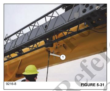
11. Connect the boom extension to the front stowage bracket by using an impact wrench and the provided extension (80104116) and socket (80104383) to turn the jack screw (1, Figure 5-31) clockwise.
