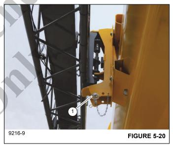
11. Disconnect the boom extension from the front stowage bracket by using an impact wrench and the provided extension (80104116) and socket (80104383) to turn the jack screw counterclockwise (1, Figure 5-21).
