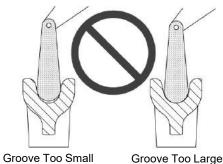
Proper fitting sheave groove should support the wire rope or 135–150° of rope circumference.
