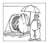
Wire ropes should be stored under cover in clean, cool and dry conditions. Contact with the ground should be avoided, e.g. by storing on pallets.
