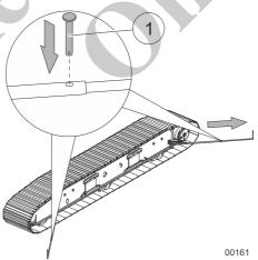
Fig. 164 Pulling out the slewing range safeguard
