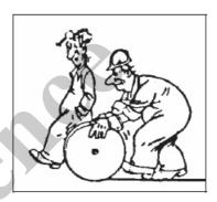
Unreeling on the ground, which is repeatedly recommended in the pertinent literature, is not very satisfactory in practice because the reel unwinds an increasingly smaller amount of rope than the distance it covers, i.e. with this approach you are forced to pull the wire rope along behind you.
