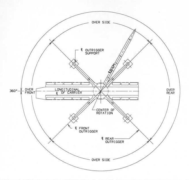
THESE LINES DETERMINE THE LIMITING POSITIONS OF ANY LOAD FOR OPERATION WITHIN THE WORKING AREAS INDICATED.
