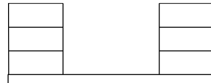
45 130 kg Crane Counterweight 6 side boxes
