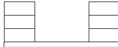
46 000 kg Crane Counterweight 6 Side Boxes
