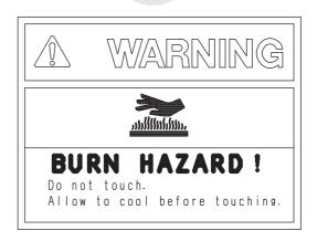
21. During engine running or straight after the engine is stopped, inside of the radiator becomes high pressure and hot.
