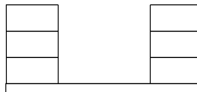
101,400 lb Crane Counterweight 6 Side Boxes
