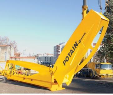
^ No bolting is required; the counter-jib can be unfolded quickly.
