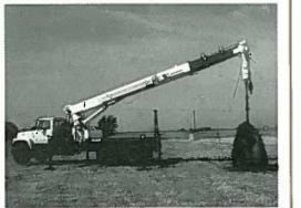
The photos at the left show the National 990 auger-equipped crane engaged in a hole-digging operation. This digging capability coupled with the Series 900's heavy-duty capacity and lofty reach, make it a remarkably versatile machine.
