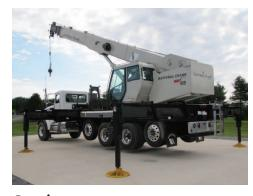
**Outriggers** Outrigger span of 7,52 m (24.7 ft) when fully extended; 5,33 m (17.5 ft) at mid-span.
