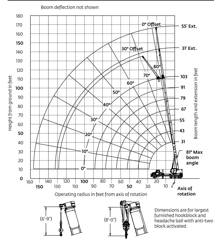
\*Drawing is to show the physical reach of the machine. Always refer to load chart to see what portions of this range are structurally and stability limited.
