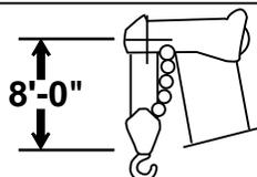
DIMENSIONS ARE FOR LARGEST GROVE FURNISHED HOOK BLOCK AND HEADACHE BALL, WITH ANTI-TWO BLOCK ACTIVATED.
