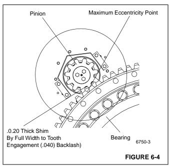
Orient ring gear such that its point of max eccentricity ("high point") is located between the swing drives. Position swing drives so that pinion is centered within cutout in base plate and motor ports face towards the outboard side as shown.
