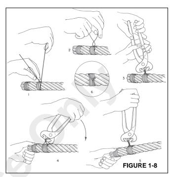
Wind a length of soft annealed wire (Figure 1-8) around the wire rope at least seven times. The two ends should be twisted together in the center of the seizing. Tighten the seizing by alternately prying and twisting. Cut off both ends of the wire and pound the twist flat against the rope.
