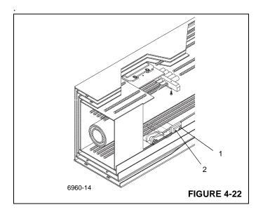
**7.** Install the bottom rear wear pad on the fly section with two screws.
