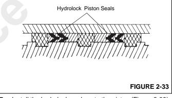
7. Install the hydrolock seals onto the piston (Figure 2-33).
