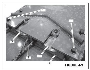
**9.** Remove the capscrews and washers (1) securing the fly retract cable anchor plates (2) to the lower front of the inner mid section. Remove the cable locknuts and the anchor plates (3) from the cables (Figure 4-10).
