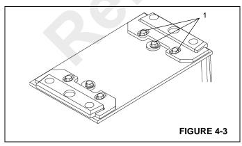
On the top front of the base section, remove the two capscrews securing each kicker plate and remove the plates.
