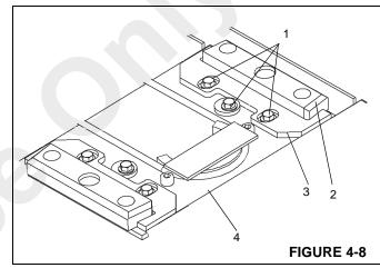
8. At the top front of the inner mid, remove the four bolts and washers (1) securing the synchronizing cable (2) sheave assembly (3). Lay the assembly with cables on top of the outer mid (4) (Figure 4-9).
