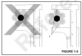
**13.** When checking for broken wires (5) (Figure 1-6) relax the rope, move it off "pick-up points", and flex it as much as possible. Use a sharp awl to pick and probe between wires and strands, lifting any wire which appears loose or moves excessively. Defect in the rope is spoke of in relations to "Lay Length" (2) which is the distance measured along rope in which one strand (3) makes one complete revolution around core (4).
