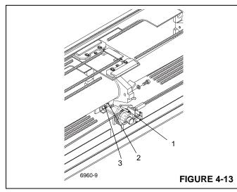
**3.** Place blocking (1) under cylinder (2) (Figure 4-14) and remove the two bolts and washers securing the cylinder barrel to the rear of the outer mid.
