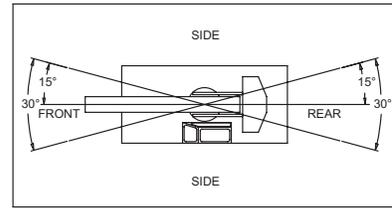
Note: For 360° rating on rubber, rear axle locks must be in place.
