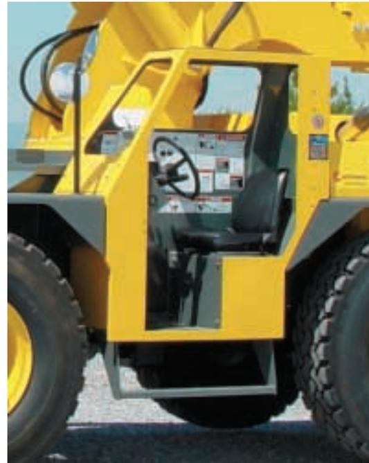
**Standard:** Open air cab shell w/overhead safety glass
