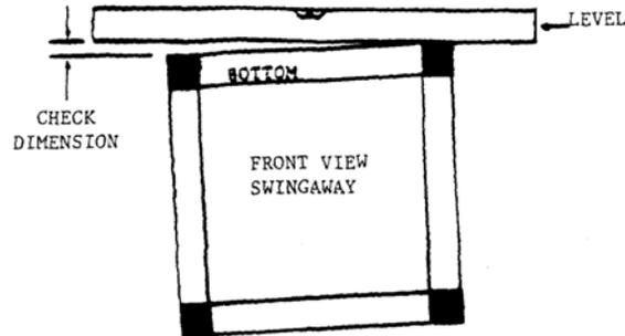
Record Check Dimension as Twist \_\_\_\_\_
