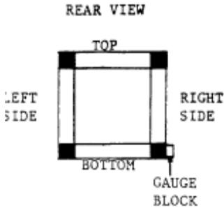
1. Checking all lacing, one side at a time, place the gauge blocks on the lacing close to the main chord.
