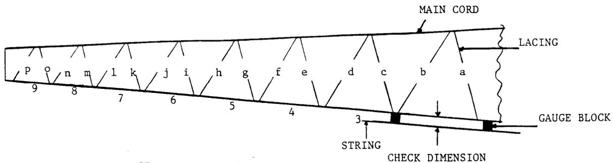
1. Place gauge blocks along outside of main chord where lacing is welded to main chord.
