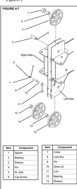
the boom with the spacer to the right hand side (Figure 4-7).
