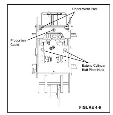
10. After the wear pads have been removed, slide the 2<sup>nd</sup>, 3<sup>rd</sup>, 4<sup>th</sup> assembly out of the 1<sup>st</sup> section and place on a suitable horizontal surface. Take care not to pinch or crush the retract cables while lifting or supporting assembly.
