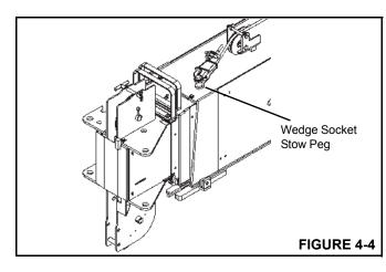
**3.** Remove the hook block or downhaul weight, wind up the rope on hoist drum, and stow the wedge socket on the pegs provided on 1<sup>st</sup> section (Figure 4-4). Shut down the truck engine.
