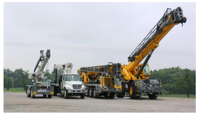
Carry Deck / Boom Truck/Truck Mount/Rough Terrain
