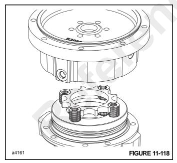
Continue disassembly removing spacer 18, friction discs 19, brake discs 20, U-cup seal 17, pressure plate 16, springs 14, and spring locator 15.
