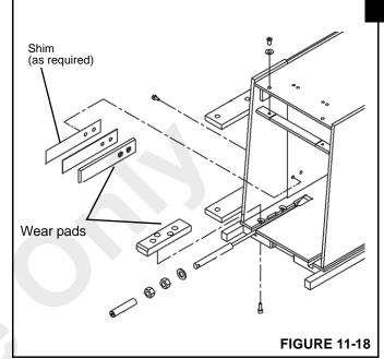
**5.** Slide the assembled sections all the way into the base section.
