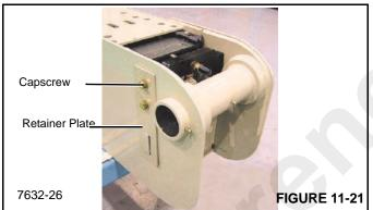
**9.** Install the retainer plates and capscrews to secure anchor plate to the outside of the base section (Figure 11-21).
