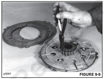
5. Wear limit of friction plates is to the depth of the crosshatching Figure 9-10. Check all plates for flatness and damage. (Wear and polishing of the counterplates is normal.) Completely replace the brake pack if worn or damaged. Do not replace individual plates.
