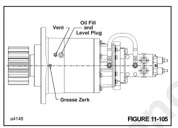
Drain the oil and clean the outside surfaces of the gearbox. Set the gearbox with the input/motor side up on a work bench and use wood blocks under the flange of the bearing carrier **2** (Figure 11-104) to stabilize it on the workbench.
