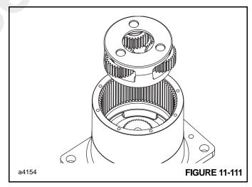
6. Remove the secondary planet carrier assembly.
