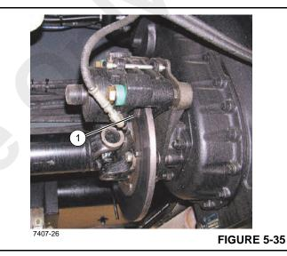
Inspect the thickness of the brake pads, Figure 5-35. Replace the brake pads if they are 7.1 mm (0.28 in) thick or less.
