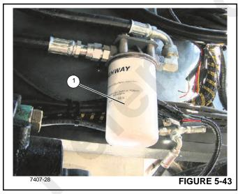
6. Coat the seal of the new filter with clean transmission oil.
