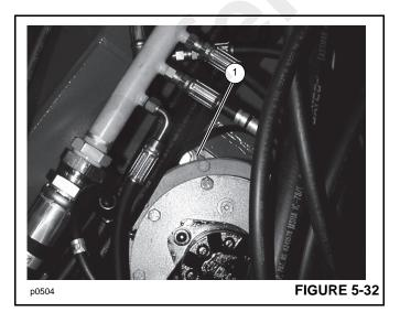
Swing Bearing to Frame Mounting Bolts
