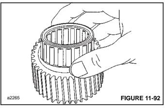
**3.** Press the remaining bushing against the race. Again, make sure the bushing is against the shoulder.
