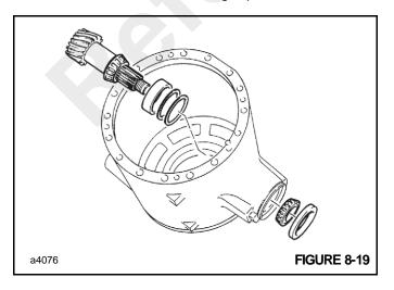
**4.** Fit the pinion inner bearing cone (Figure 8-20) and a new collapsible spacer.
