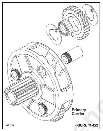
**NOTE:** The primary planet carrier assembly has one row of loose roller bearings under the planet gears, while the output carrier has two rows of loose rollers under each gear.
