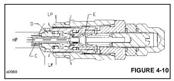
The imbalance of pressure on the inside as compared to that of the high pressure port "HP" forces the relief valve poppet "D" (Figure 4-11) to open and relieve the oil directly to the low
