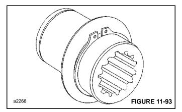
5. Slide the inner race through the bushings and sprag clutch. The race will have to be rotated in the freewheeling direction to start it through the sprag clutch. If the inner race will not go through the bushings, the bushings have probably been damaged and should be replaced.
