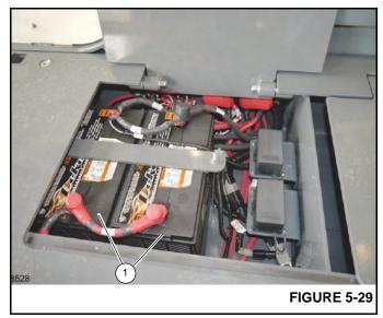
6. Coat the battery posts with petroleum jelly and reinstall the battery cables.
