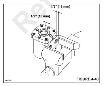
**11.** Remove four capscrews **1** from mounting flange **3**. These screws were installed with Loctite to hold them in place.
