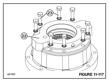
The force of the brake springs is applied to the motor adapter 22, so loosen the metric capscrews 23 one turn at a time, alternating across the gearbox, until the spring force is released. Remove the motor adapter and discard O-ring 21.
