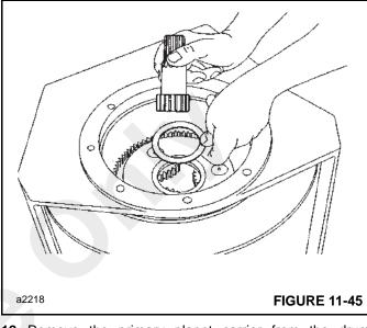
**12.** Remove the primary planet carrier from the drum (Figure 11-46). Refer to *Planet Carrier Service, page 11-28* for additional information.
