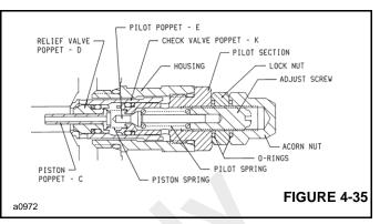
To perform service, clean the surrounding area and remove the complete relief valve cartridge. Examine the seat in the main relief housing and if grooves and ridges are evident, the valve must be replaced.
