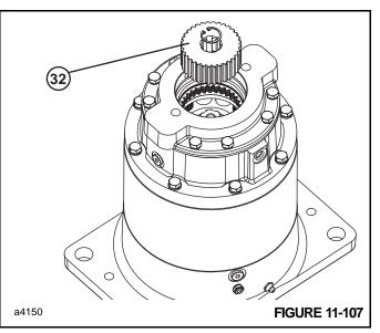
2. Disconnect the brake release hose at the gearbox. Unbolt and remove the hydraulic motor from the gearbox. Remove the brake hub 32 and remove and discard the motor pilot O-ring.
