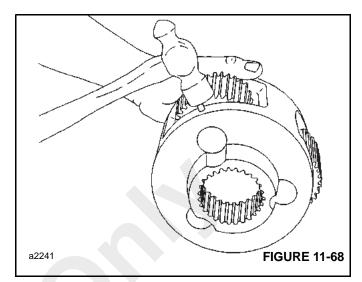
4. Note that the roll pin is slightly recessed in the carrier when properly installed. With a center punch (Figure 11-69); stake the carrier next to the pin hole as shown. This will distort the hole so the pin will not back out. Repeat these steps for each of the three planet gears.
