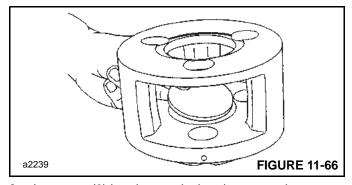
Insert two (2) bearings and a bearing spacer into a gear with the spacer between the bearings. Place a thrust washer on each side of the gear and position in a carrier opening. Slide the shaft through the carrier, thrust washer, bearing gear subassembly and remaining thrust washer (Figure 11-67).
