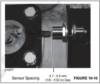
2. Measure the distance between the end of the sensor and edge of the sensor bracket. The sensor spacing must be between 3.3 mm (1/8 inch) to 5.6 mm (7/32 inch). If the spacing is incorrect, adjust the spacing with the jam nuts on the sensor. Be sure they are tightened after proper gap is obtained.
