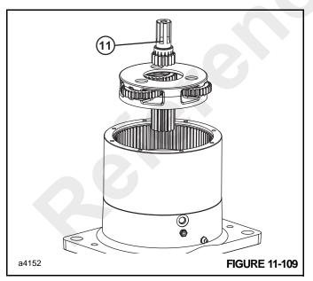
Remove the primary sun gear 11 and the thrust washer 31.
