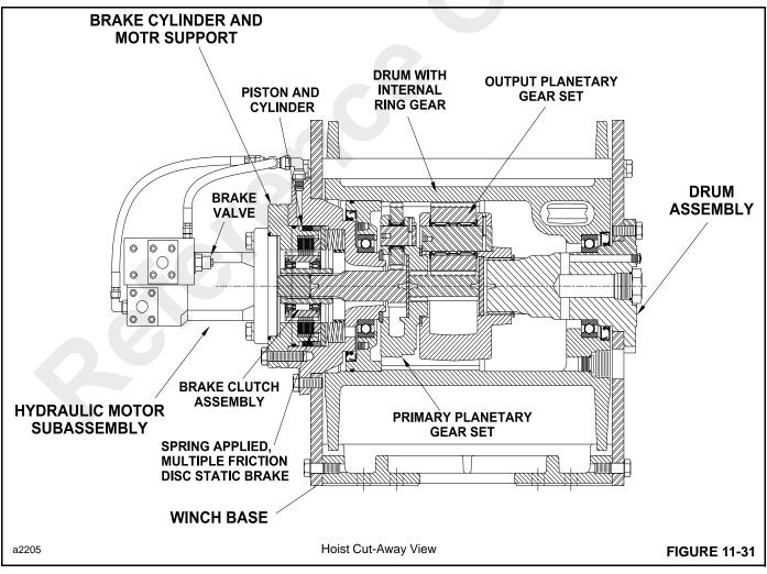
The primary planet carrier drives the output planet sun gear, which in turn drives the planet gears. The output planet carrier is splined to the bearing support and cannot rotate. Therefore, as the output planet gears are driven by the sun gear, they will drive the ring gear/drum.
