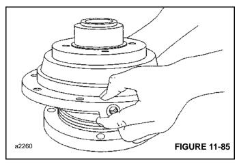
**9.** Install the motor support capscrews and tighten evenly to recommended torque.
