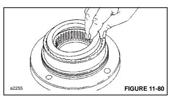
4. To check brake stack height, place a pressure plate on top of brake spacer. Hold pressure plate down firmly by
