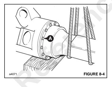
**3.** Separate the axle arm from the drive head (Figure 8-5) by tapping the flange with a soft faced hammer. Remove all traces of gasket material from the mating faces.
