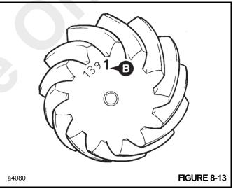
If dimension **B** is positive, add it to the bearing depth. If 4. dimension **B** is negative, subtract it from the bearing depth.
