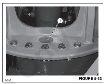
Mast to Swing Bearing Mounting Bolts
