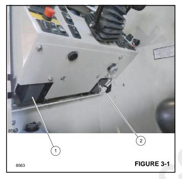
The main fuse/relay panel (1, Figure 3-1 and Figure 3-2) is located below the left side of the dash. Refer to Figure 3-2 for identification of the relays and TABLE 3-1 for identification of the fuses.
