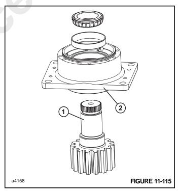
10. Remove output pinion from bearing carrier 2.
