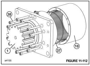
If the output pinion 1 will be removed, remove the ring gear 10 from the bearing carrier by removing the metric socket head capscrews 38 and discard the ring gear Orings 37.
