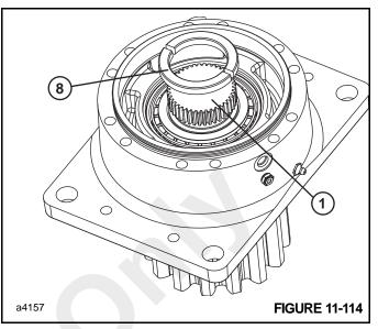
**9.** Take care not to damage the ground surface of the split ring halves. Use a hammer and punch to remove the split ring halves **8** from the output pinion **1**.
