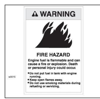
Maintain control of the hose nozzle when filling the fuel tank. Do not allow fuel to spill. Clean up spilled fuel immediately. Dispose of clean up materials properly.
