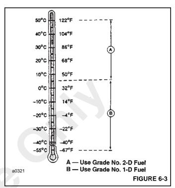
**NOTE:** If engine is operating at temperatures of -40° to -57°C (-40° to -70°F), Grade DF-A arctic fuel is recommended. Also consult the engine distributor for special lubricants and starting aids.
