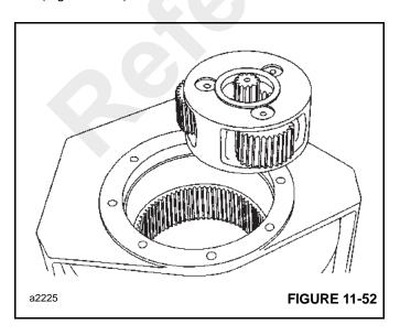
**7.** Install the output planet carrier (Figure 11-53) into the drum while meshing the planet gears with the ring gear and the planet housing with the bearing support.
