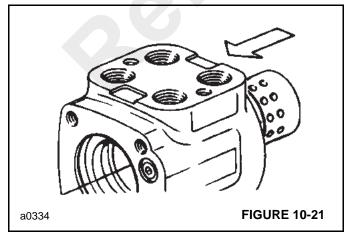
**NOTE:** Be extremely careful that the parts do not tilt out of position while inserting. Push parts gently into place with a slight rotation action; keep the pin
