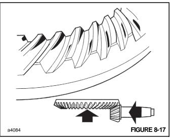
**NOTE:** The crownwheel and pinion are matched and should be renewed as a pair if either one is damaged or excessively worn.
