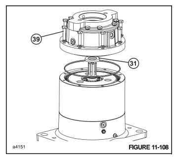
**3.** Remove the complete brake cylinder assembly by removing the eight metric bolts **39** and lifting the brake cylinder off of the ring gear. See *Brake Cylinder Service, page 11-48* for procedure to disassemble the brake cylinder assembly.
