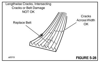
Any ribbed belt showing signs of wear or that has material missing should be replaced. When a belt is replaced, check its tension again after 30 minutes of operation. New belts will stretch with use.
