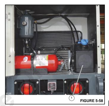
This engine uses a Selective Catalytic Reduction (SCR) system. SCR is a technology that uses a urea based DEF and a catalytic converter to significantly reduce oxides of nitrogen (NOx) emissions.
