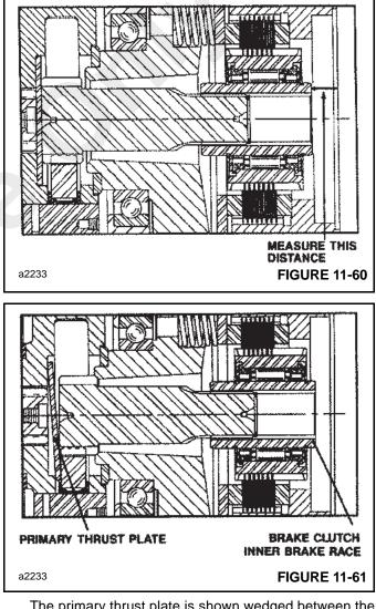
The primary thrust plate is shown wedged between the planet gears and the planet carrier. Note that the primary sun gear and the entire brake clutch assembly have moved to the right (toward the hydraulic motor).
