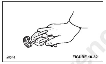
**c.** Locate the seal in the end cap groove (Figure 10-33). When the seal is in position, open the tool to release the seal. Make sure the seal is correctly installed in its groove then remove the tool.
