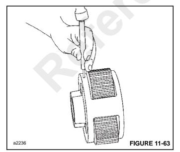
**2.** Use a punch (Figure 11-64) to drive the roll pins from the planet shafts. Do not reuse the roll pins.
