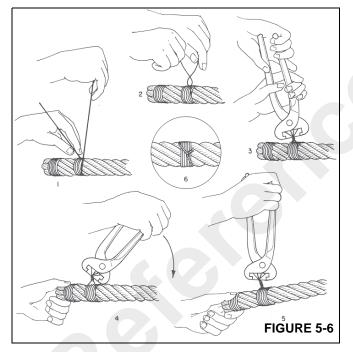
Wind a length of soft annealed wire (Figure 5-6) around the wire rope at least seven times. The two ends should be twisted together in the center of the seizing. Tighten the seizing by alternately prying and twisting. Cut off both ends of the wire and pound the twist flat against the rope.
