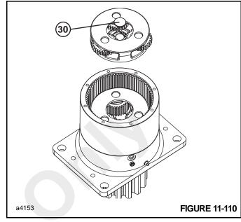
**5.** Remove the primary planet carrier assembly and thrust plug **30**.
