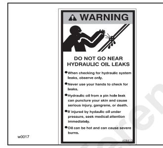
Inspect hydraulic hose assemblies for leaks, damaged fittings and worn exterior. Do not use your hands to check for hydraulic leaks. Hydraulic oil under pressure can cause serious injury or possible death. Use a piece of cardboard or other material as a deflector to detect leaks. Replace any problem hose before beginning work.
