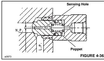
If operating difficulties indicate that the pilot poppet is leaking or sticking, remove internal parts of the pilot section, and follow the same procedure as above. After assembly, adjust the relief valve pressure per instructions in this section.
