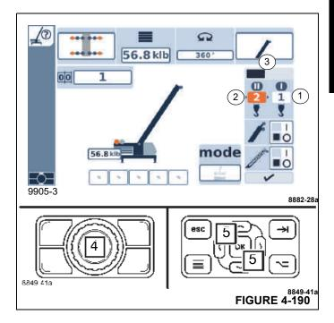
Position the slider bar (3, Figure 4-190) over the top of the hoist that is to be used. Example screenshot in Figure 4-190 shows the Auxiliary Hoist is selected.
