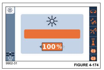
Press the Jog Dial or OK Button on the Navigation Control Pad, then use the Jog Dial or Arrow Buttons to increase or decrease the screen brightness. Once the desired value is selected, press the Jog Dial or OK Button to accept the value.
