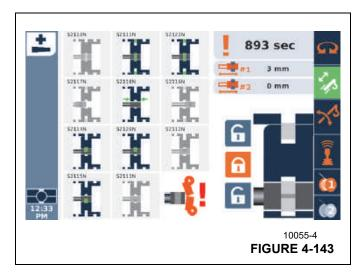
In this triggered condition, the telescoping cylinder is no longer expected to be able to extend. If the extended emergency telescoping mode is being used, then it is possible to still extend the cylinder (such as when the switch is malfunctioning or disconnected), but this should only be done with physical verification of the location of the telescoping cylinder with respect to the boom nose. If the telescoping cylinder impacts the boom nose, the boom system will be damaged.
