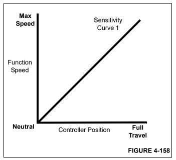
Selecting a sensitivity curve of 2 through 5 causes the function speed to be reduced, from the default sensitivity curve 1, relative to the same controller position over the full travel of the controller (Figure 4-159).
