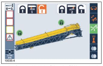
**b.** Press and hold the OK on the ODM control pad or press down on the jog dial.
