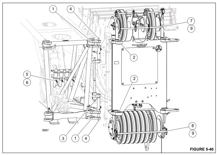
10. Remove pins (5, Figure 5-40) and retaining clips (6) from the stowage bracket. Secure the boom extension to the boom nose using four pins (5). Secure the pins (5) with retaining clips (6). If necessary, remove the upper (7) and lower (8) hoist rope rods and retaining clips (9) to install the pins (5). Use the jack as necessary to install the fourth pin as necessary as follows:
