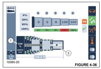
The example in Figure 4-36 shows the value of 10571 mm for the extension of the telescoping cylinder within the boom. This is the value from the precision length sensor. The example also shows a value of 108.8 feet as the overall boom length. The example shows the T5 boom section had been previously extended and locked at its 100% pinning location and the T5 boom section is being pinned at the 100% pinning location. The remaining boom sections are locked at their 0% pinning location.
