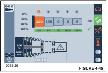
Typically shut-down condition indicates a failure in the components of the control system (such as sensors or modules or communications). If the only indication of faults is for the telescoping function, then the following steps can be used:
