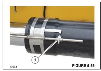
6. In the ODM, verify that the front (Pin #2) and rear (Pin #1) boom extension pins are securely installed. Visually confirm that the pins are installed.
