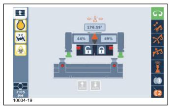
When the counterweight cylinders are fully retracted, the counterweight is removed.
