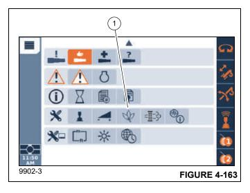
The Economy (ECO) Mode function offers the operator a convenient way to reduce noise and fuel consumption during craning operation. ECO Mode does this by automatically increasing the engine speed to an operator specified engine working speed when craning functions are operated and then decreasing the engine speed to idle speeds when no craning functions are operated.
