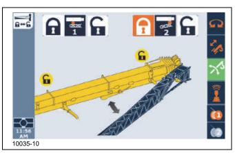
**b.** Press and hold the OK on the ODM control pad or press down on the jog dial.
