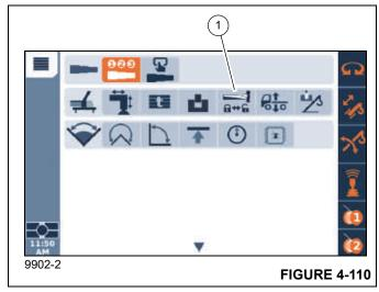
The Boom Extension Deployment/Stowage function screen is used to extend and retract the front and rear boom extension pins that secure the boom extension to the boom base section.
