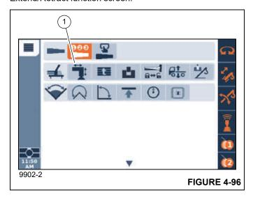
The Outrigger Extend/Retract function screen (Figure 4-97) allows the operator to set the outriggers and level the crane using either a manual or semi-automatic mode. The outriggers are also retracted and stowed from this function screen.
