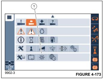
The Display Screen Brightness function screen (Figure 4-174) allows the operator to adjust the brightness of the ODM and RDM display screens.
