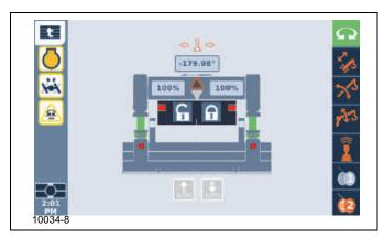
c. The superstructure swings the cylinders out of the counterweight mounting posts.
