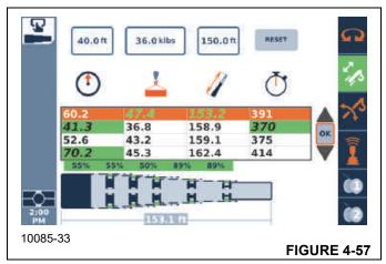
Finally, if it is desired to keep lifts within a criterion such as 75% of the maximum values for the load chart data, then the search can be based on a modified hook load. The modified hook load value would be the hook load divided by the decimal value for the desired limitation such as the following:
