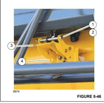
**11.** In the ODM, highlight the unlock icon and the retract the rear boom extension pin (Pin #1) as follows:
