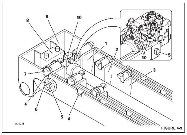
Each telescopic section is equipped with two section locking pins (7) which are extended by spring force.
