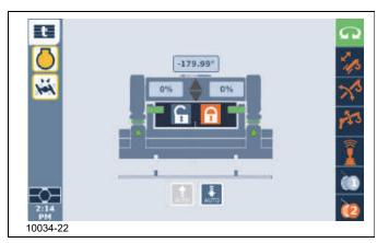
When the locking pins are locked, the counterweight is installed.
