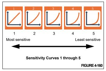
Adjust the sensitivity of a controller function by doing the following:
