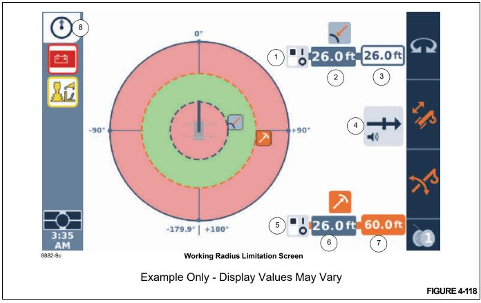
Using the Left Arrow and Right Arrow function on the display or the jog dial changes the Icon highlighted on the screen. As the Icons, with the color orange typically meaning that the Icon is selected and can be affected by subsequent actions.
