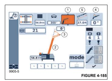
Use symbol (1, Figure 4-185) to select the rigged boom system.
