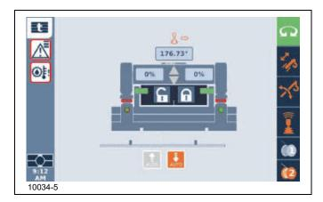
**NOTE:** If two direction arrows appear, it means the controller can be moved in either direction.
