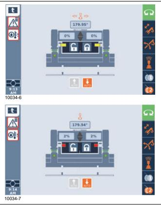
**b.** The lift cylinders lower the counterweight to the carrier platform. The progress of the cylinders is shown in percent. The cylinders are fully retracted when 0% is displayed. The cylinders are fully extended when 100% is displayed.
