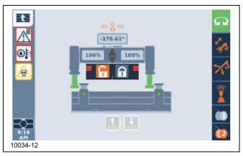
**b.** The superstructure swings the cylinders in to the counterweight mounting posts.
