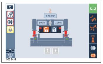
**d.** When the lift cylinders are fully retracted (0%), release the controller. When the cylinders are fully retracted, the counterweight is installed on the carrier platform.
