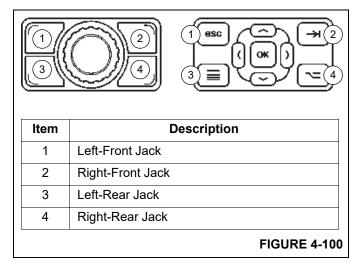
When a button at the Jog Dial or Navigation Control Pad is pressed and held, the corresponding O/R jack image turns orange to indicate that it is actively moving. An arrow
