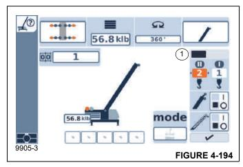
To switch between main hoist or auxiliary hoist, refer to Example of how to Switch over the Hoists, page 4-165.
