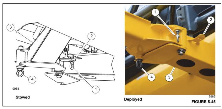
**10.** Remove retaining clip and pin (1 and 2, Figure 5-46) from holes in the fly section stowage bracket (3). Install the retaining clip and pin in the storage position (4).
