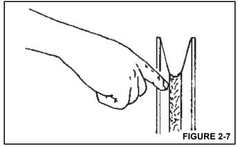
Inspect the boom nose and hook block sheaves for proper operation, excessive wear, and damage every 50 hours or weekly. Inoperable, damaged and/or worn sheaves cause rapid deterioration of rope.
