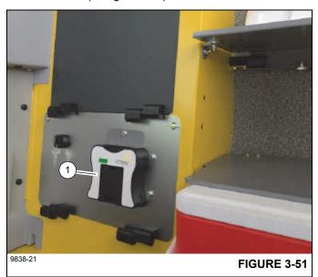
The charger is always on and will charge the battery pack whether the engine is operating or not.
