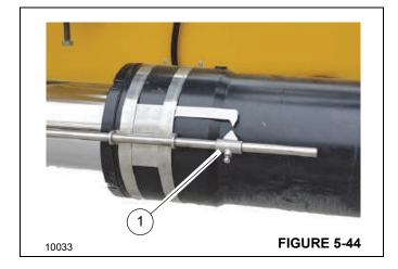
In the ODM, verify that the front and rear mounting pins are securely installed. Visually confirm that the pins are installed.
