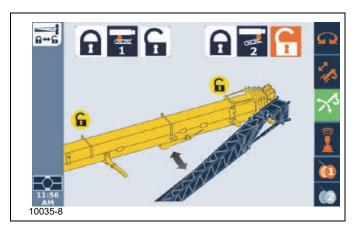
**a.** Use the ODM control pad arrow buttons or jog dial to highlight the Pin #2 lock icon.
