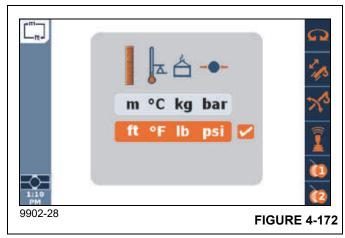
Use the Jog Dial or Arrow Buttons on the Navigation Control Pad to select the desired unit of measure, then press the Jog Dial or the OK Button to accept the new setting.
