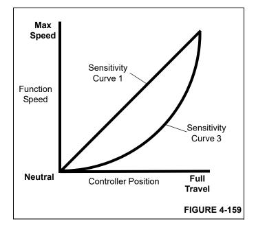
Sensitivity curve 1 (default) is the most sensitive and sensitivity curve 5 is the least sensitive (Figure 4-160).
