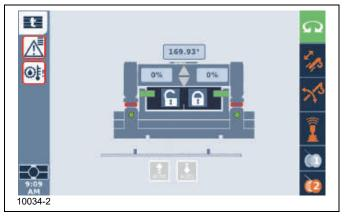
**6.** Rotate the superstructure so the rear is over the counterweight platform on the front of the carrier. When within range, the Auto icon becomes active. The valid range to activate Automatic mode is -176.5° to 176.5°.
