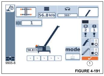
The Monitoring menu is opened and the rigging code is applied.
