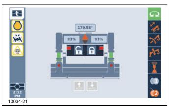
**13.** Using the ODM navigation control pad or jog dial, highlight the lock icon <a>▶</a>. Press and hold the OK button on the ODM navigation control pad or the jog dial until the locking pins are locked (green).
