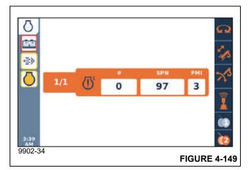
If several fault codes are active, use the Jog Dial or Arrow Buttons on the Navigation Control Pad to select the arrow at the top or bottom of the screen to scroll through the codes
