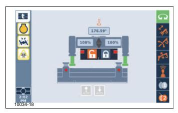
**14.** Using the ODM keypad or jog dial, highlight the Up arrow . Press and hold the OK button on the ODM navigation control pad or the jog dial down until the counterweight cylinders are fully retracted.
