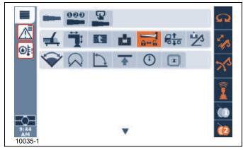
Press the OK button on the ODM navigation pad or press down on the jog dial to select the Boom Extension Deployment/Stowage icon.
