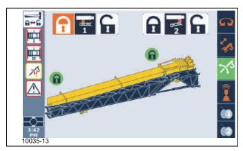
**15.** Visually confirm that the front boom extension pin (Pin #2 in the ODM) is locked. The handle should be in the up position. When the handle is in the up position, the front mounting pin is extended and the boom installation pins are unlocked. Lock the handle (1, Figure 5-38) with pin (2).
