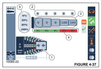
The arrows (1, Figure 4-37), at some point in the telescoping process, will blink. The blinking is an indication that an unlocking or locking event will occur if the operator holds the joystick in the direction of that arrow for at least 1 second. If this event begins, then the screen will change to the dots (as described for Figure 4-36) so that the operator knows that an automated motion or action is again occurring.
