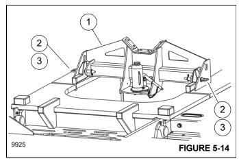
**5.** Remove the lift cylinder support (1, Figure 5-14) from the counterweight platform as follows:
