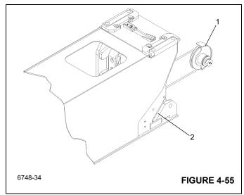
17. Lubricate the retract cable shaft.
