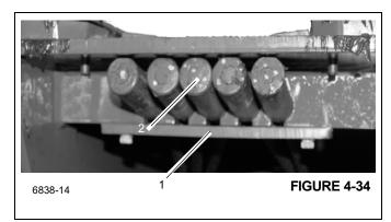
4. After supporting the weight of the telescope cylinder, remove the two bolts securing the cylinder foot weldment (1), (Figure 4-35) to the telescope cylinder (2), (Figure 4-35). Remove the foot weldment.
