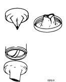
Vacuator valves are designed to expel loose dust and dirt from the air cleaner body automatically, thus lengthening the element service life. The valve lips must point straight down and be kept free from debris to operate effectively. Mud and chaff can lodge in these lips periodically and hold them open during engine operation.
