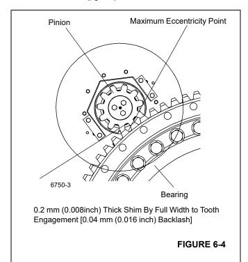
Orient ring gear to the point of max eccentricity ("high point"). Position swing drive so that pinion is centered within cutout in base plate and the motor ports face towards the outboard side as shown in (Figure 6-4).
