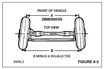
0.794mm (1/32 inch)  $\pm$  0.794mm (1/32 inch) for Loaded vehicle.
