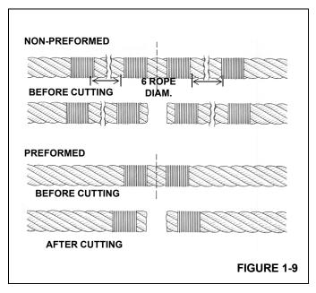
**Installing 35x7Class Wire Rope**
