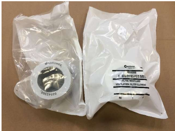
1x 03142360 Chassis hydraulic oil tank ventilation filter
